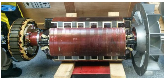
Fig. 8. The rotor of the experimental exciter being tested, with the rotating diode bridge feeding the rotor of the main synchronous generator.
