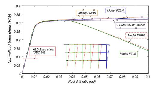
Figure 4. LA3 building - Nonlinear static (pushover) capacity curve considering a  $1^{st}$  mode lateral load pattern
