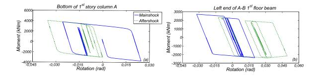
Figure 8. LA3 building hinge moment-rotation response at: (a) bottom of first story in grid line A; (b) left end of first floor level beam A-B
