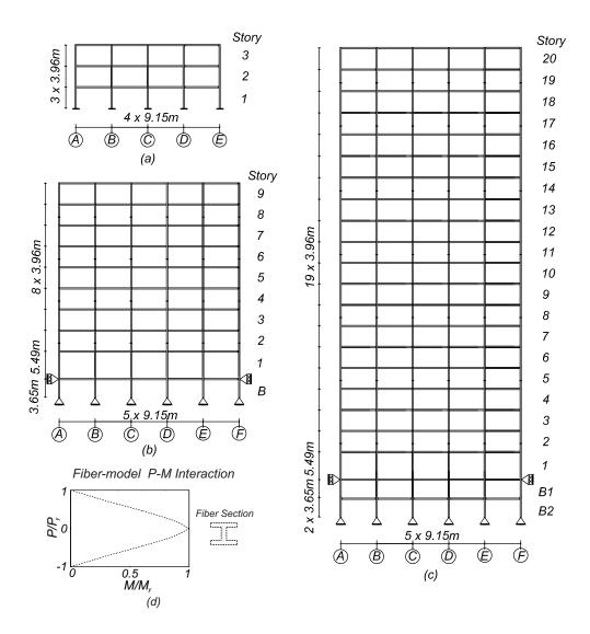
Figure 2. Building Models (a) LA3; (b) LA9; (c) LA20; and (d) P-M interaction curve
