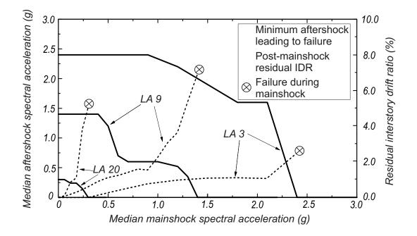
Figure 12. Median lowest aftershock ground motion spectral acceleration at the fundamental period of the intact structure that leads to failure (solid line and left vertical axis) and median residual interstory drift ratio after mainshock (dashed line and right vertical axis) as a function of the median mainshock ground motion spectral acceleration
