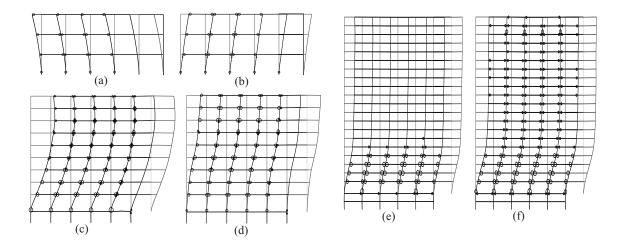
Figure 9. Deformed shapes of the buildings at two different instants: (a,c,d) - Peak interstory drift ratio during the mainshock; and (b,d,f) - Peak interstory drift ratio during the aftershock, for LA3, LA9 and LA20, respectively.
