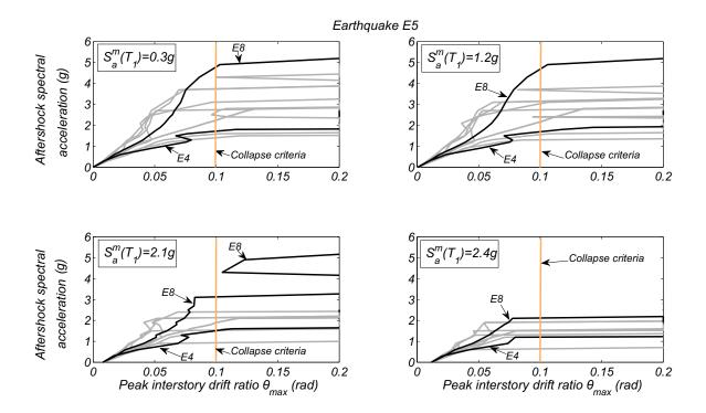
Figure 10. LA3 building - Aftershock IDA curves for ten earthquake records and four different mainshock ground motion spectral accelerations
