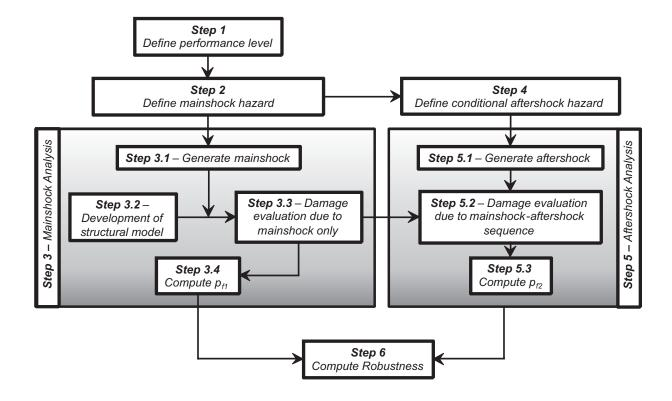
Figure 1. Flowchart for the robustness assessment of buildings subjected to cascading seismic events
