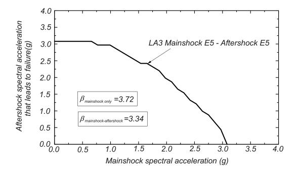
Figure 11. LA3 building - Aftershock ground motion spectral acceleration at the fundamental period of the intact structure that leads to failure as a function of the mainshock ground motion spectral acceleration for earthquake E5
