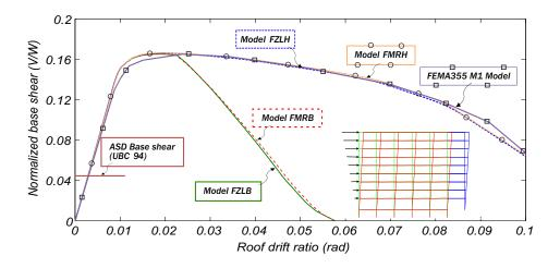
Figure 5. LA9 building - Nonlinear static (pushover) capacity curve considering a  $1^{st}$  mode lateral load pattern
