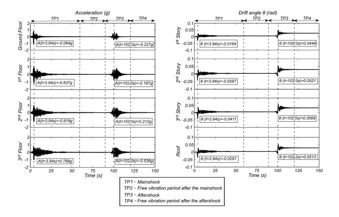
Figure 7. LA3 building - Example of a mainshock-aftershock back-to-back acceleration and drift response time-histories
