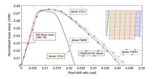
Figure 6. LA20 building - Nonlinear static (pushover) capacity curve considering a  $1^{st}$  mode lateral load pattern
