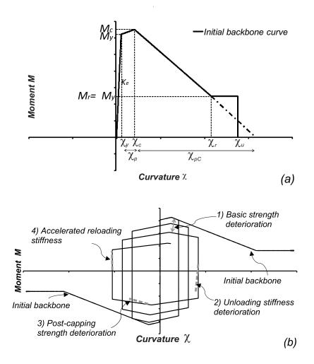
Figure 3. Adapted modified Ibarra-Krawinkler model: (a) backbone curve; and (b) basic modes of cyclic deterioration
