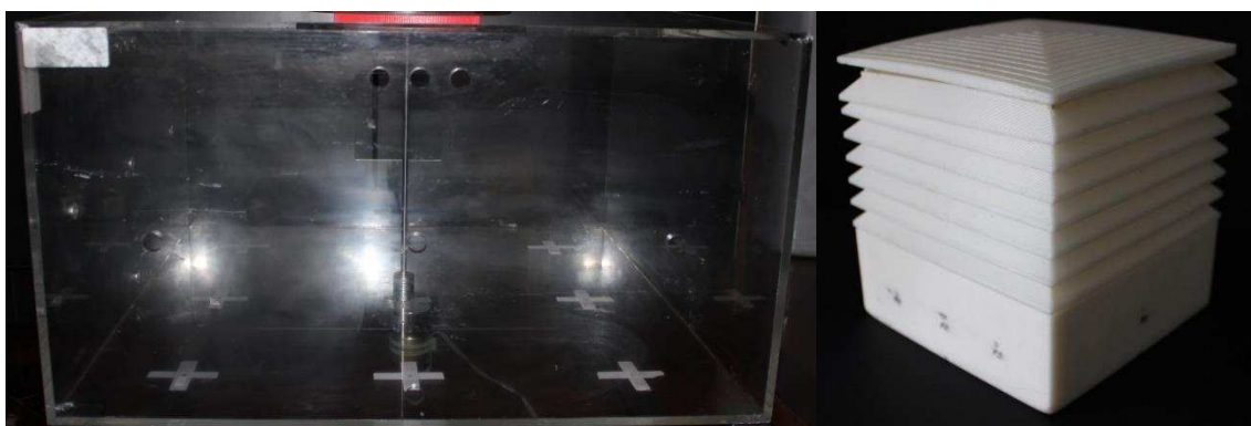
Figure 6 –Building model (left) and standard wind tower (right) used in wind tunnel experiments. Exact copies were produced for use in CFD analysis
