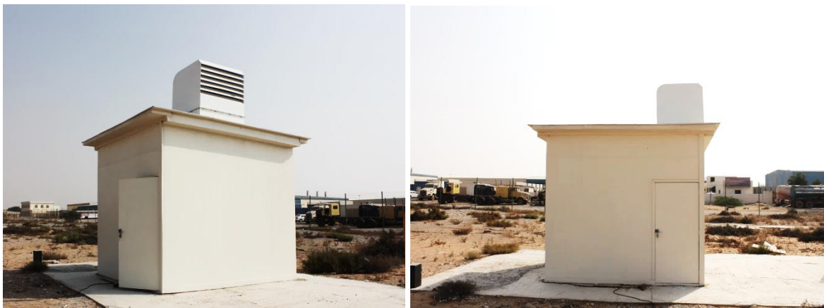
Figure 11 (a) Isometric view and (b) side view of the windcatcher mounted on top of the test room.
