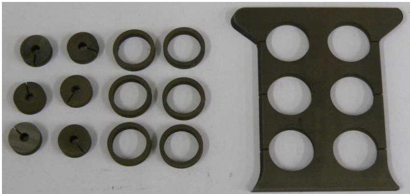
Figure 9: Ring specimens and remains from EDM operations.
