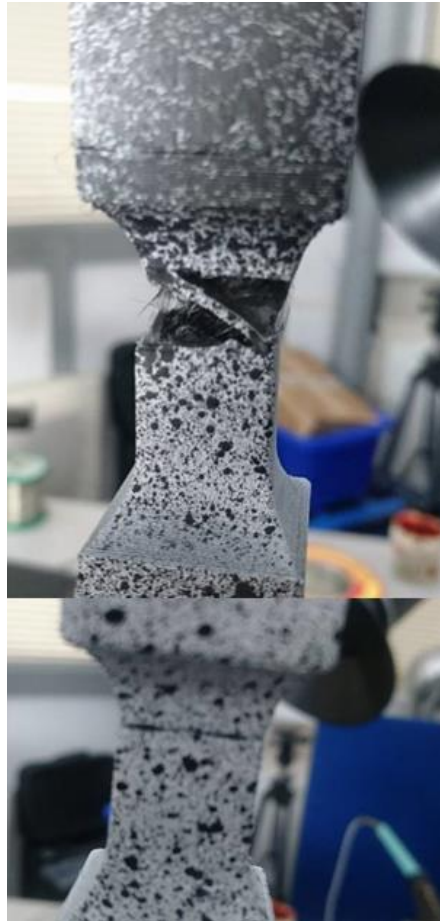
Figure 11: The fracture interface of Sets 2 and 3. The top photo shows carbon fibre being stretched during testing, suggesting the fibre assisted in resisting tension
