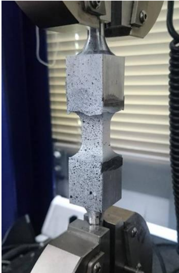
Figure 6: Through-thickness tensile specimen with fitted end-tabs and texture spray paint ready for testing.
