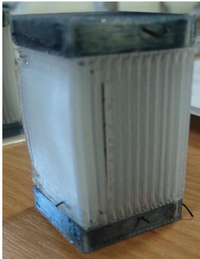
Figure 9: Set 4 specimen with CF splinters
