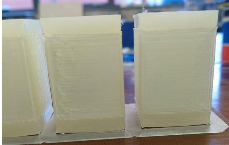
Figure 7: Thermal distortion in original Set 1 specimens.
