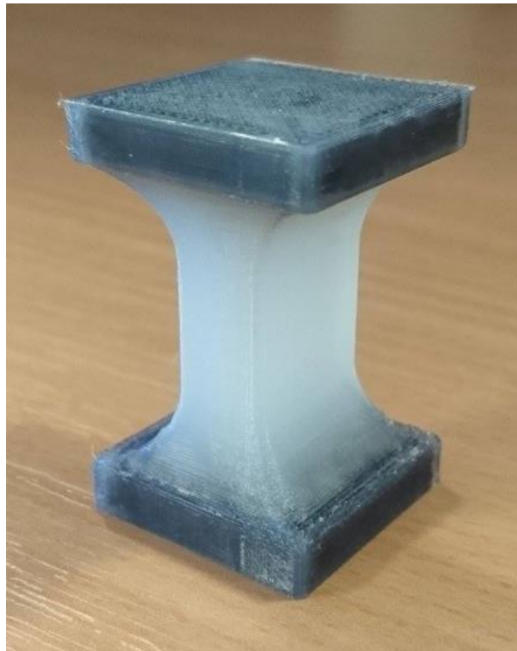
Figure 8: Set 1 (0% carbon fibre) specimen with reinforced bases.
