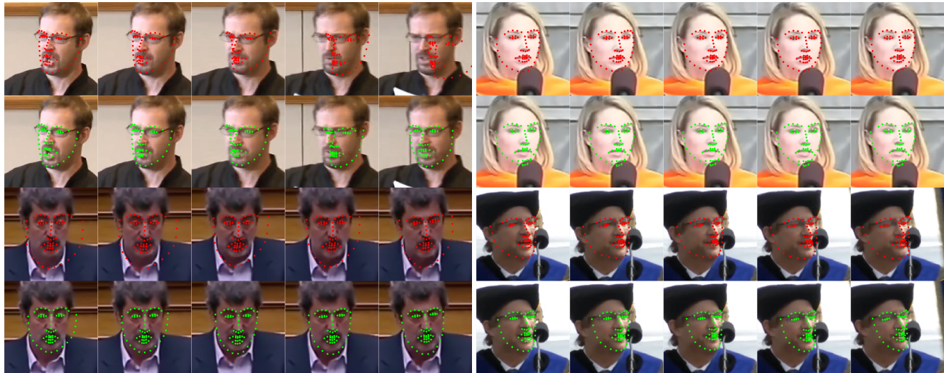
Fig. 9. Visual examples from Category 3 on 300VW. Upper rows show the CCR fitting (red points), whereas the lower rows show the iCCR fitting (green points). The sequences on the left show a clear case where iCCR outperforms CCR thanks to its incremental learning capabilities (fast movement in the upper sequence, low resolution in the sequence at the bottom). The sequences on the right show a failure case where the learned features are not capable to outperform CCR. All qualitative videos and results can be found at https://continuousregression.wordpress.com/code .
