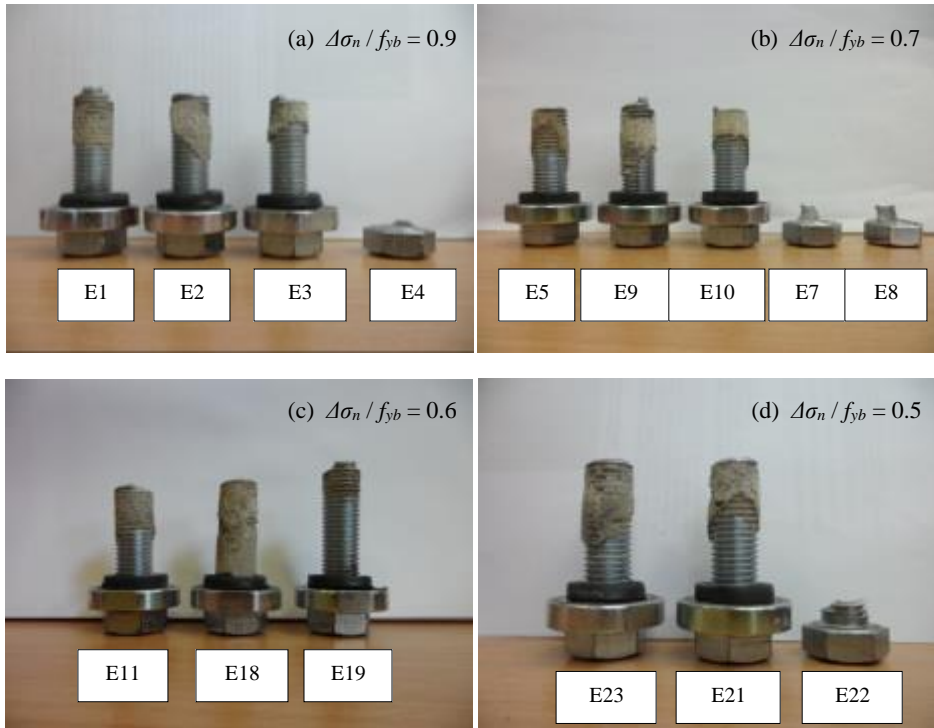
Fig. 9. Failure mode of Extended Holo-bolt
