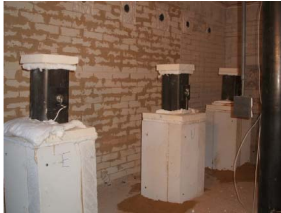
Fig. 4. Location of test specimens in furnace.
