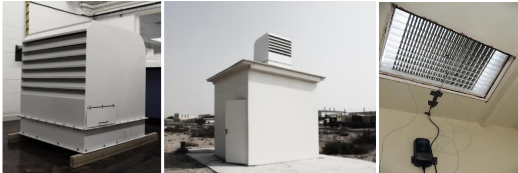
Fig. 3. (a) Full scale windcatcher prototype; (b) windcatcher installation; (c) measurement of supply air
