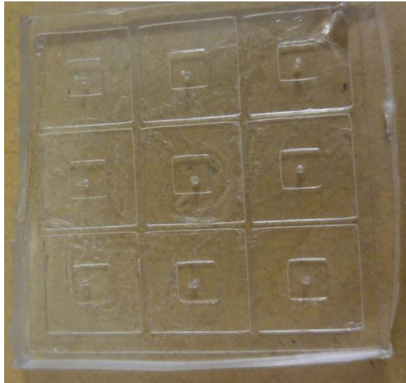
Figure 5-5: Fabricated Device with Patterns to Test Bond Strength
