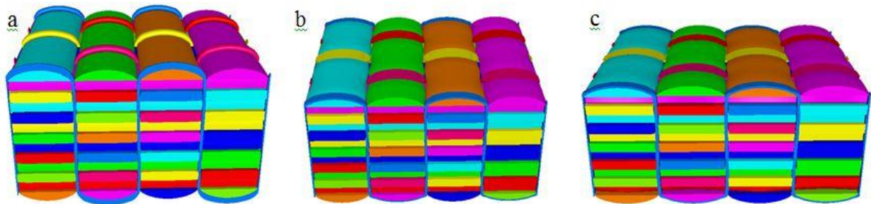
Figure 3. Orthogonal weave generated using 3DWizard refine option. (a) original fabric thickness, 6.315 mm; (b) fabric thickness 5.03 mm; (c) fabric thickness 4.432 mm.
