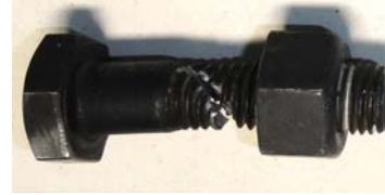
(f) Fractured bolt in specimen SJST
