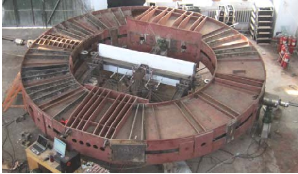
Fig. 5 Multifunctional loading ring
