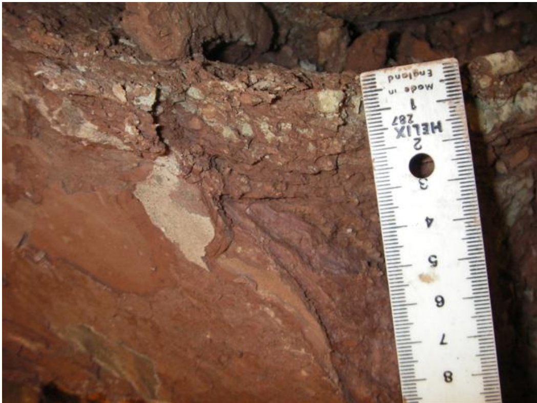
Figure 4.37 The remoulded zone from around pile MR3 860-1210mm below ground level taken from above
