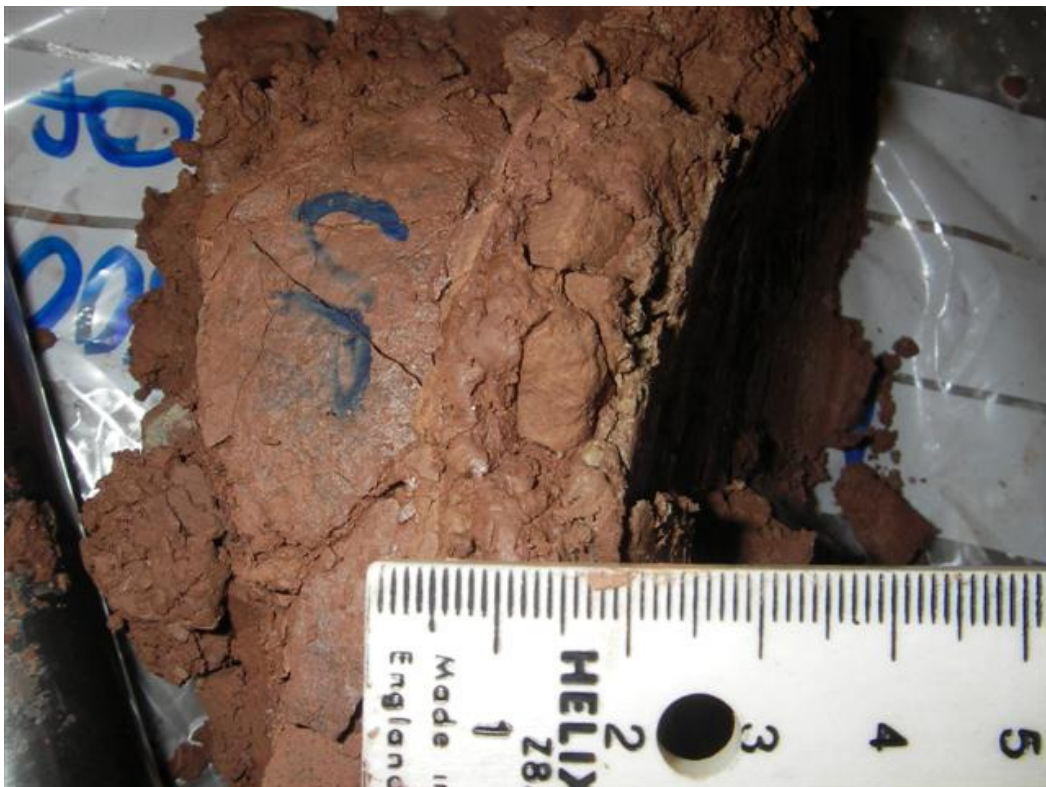
Figure 4.36 The remoulded and undisturbed material from pile MR3 860-1210mm below ground level looking down from above
