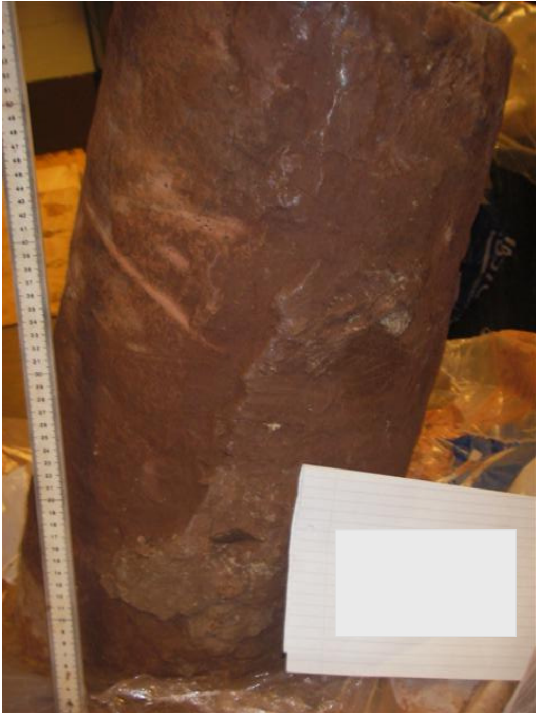
Figure 4.29 The fourth section from pile MR3 1210-1831mm below ground level
