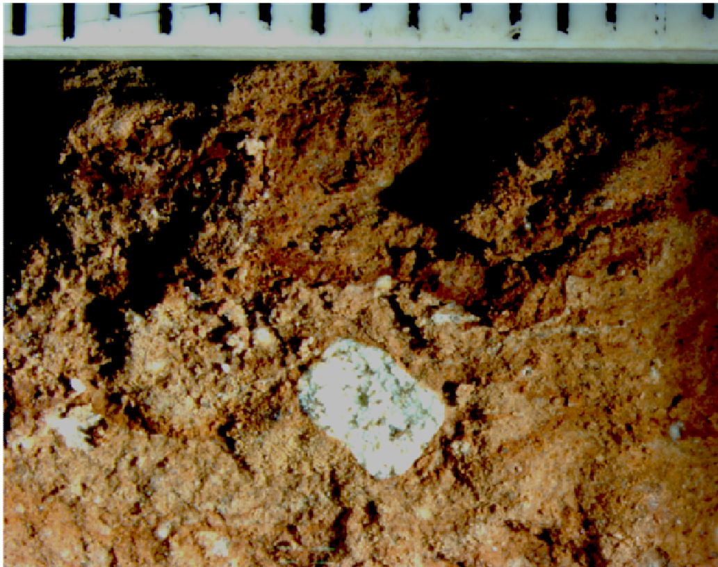
Figure 4.47 Sample taken from the remoulded zone surrounding MR2 690-1000mm below ground level, ruler shows the original location of the pile. Photograph is taken from above; increments indicate lengths of 1mm.
