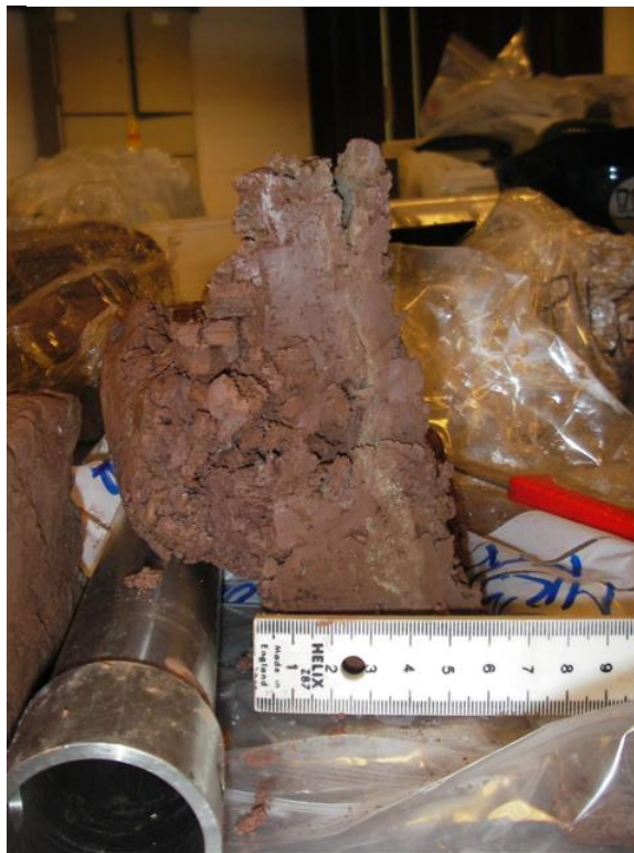
Figure 4.35 Zoning within the remoulded zone of pile MR3 at 860-1210mm below ground level, pile would have been at the right of this photograph
