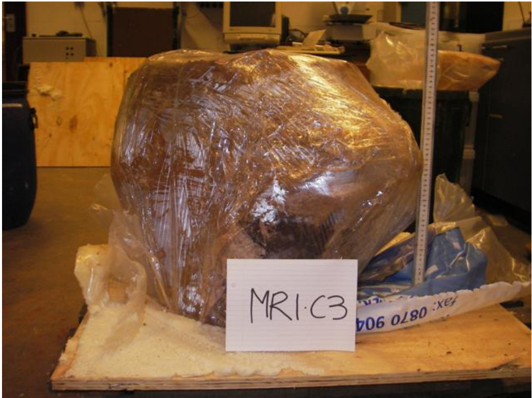
Figure 4.11 The section from pile MR1 819-1277mm below ground level
