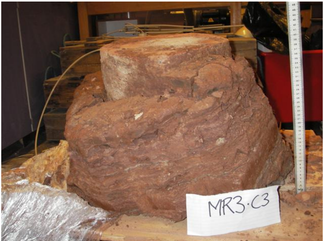
Figure 4.28 The third section from pile MR3 860-1210mm below ground level
