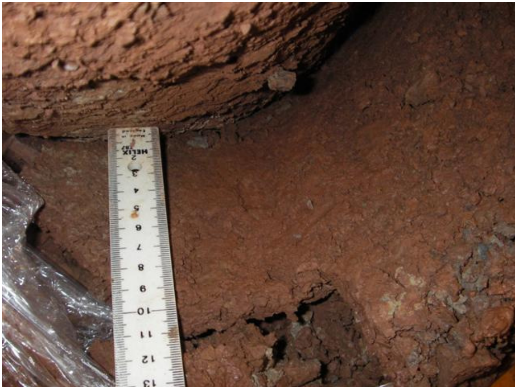
Figure 4.31 The boundary between remoulded and undisturbed material from the soil surrounding pile MR3 510-860mm below ground level
