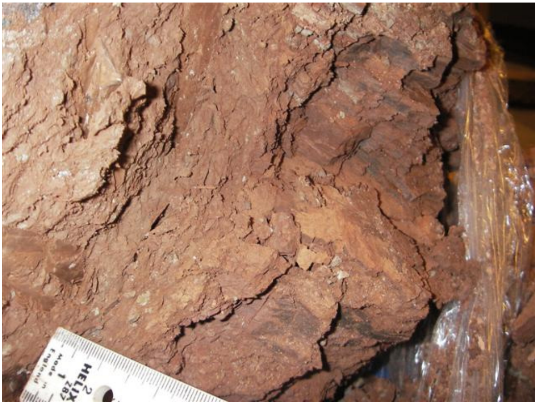
Figure 4.22 A vertical section through the remoulded zone of pile MR2 1000-1457mm below ground level. Photograph shows remoulded and undisturbed material
