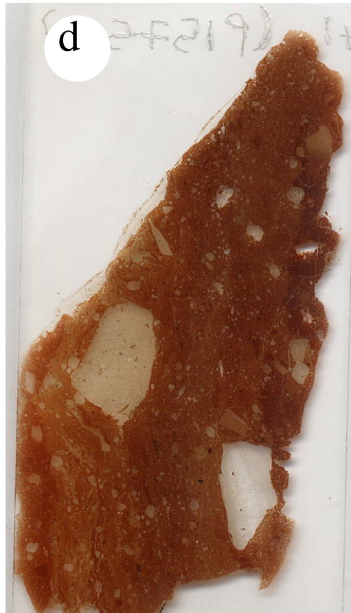
Figure 4.56 Horizontally taken slides from around all four piles) MR1, slide is 19mm wide b) MR2, slide is 17mm wide c) MR3, slide is 48mm wide d) MR4, slide is 40mm wide. In all cases except photo c the pile is to the right of the picture. In the case of photo c the pile is to the bottom of the picture.
