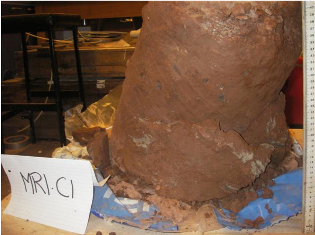
Figure 4.9 The section from pile MR1 0-495mm below ground level
