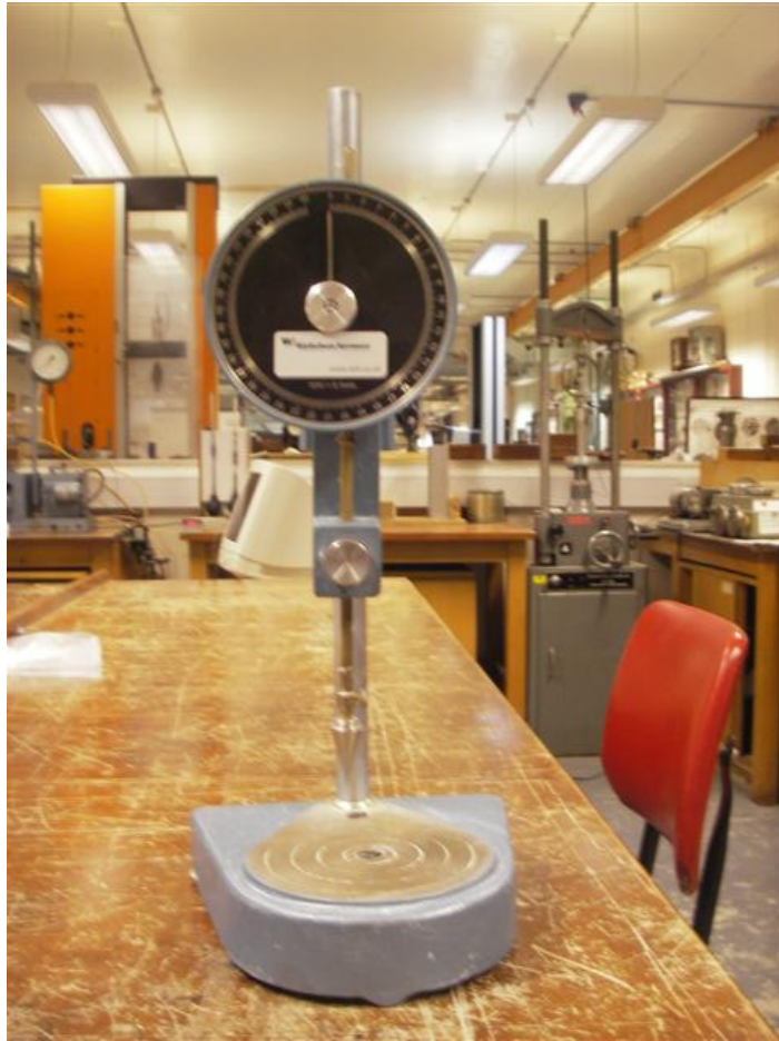
Figure 3.15 The cone penetrometer equipment used in liquid limit experiments
