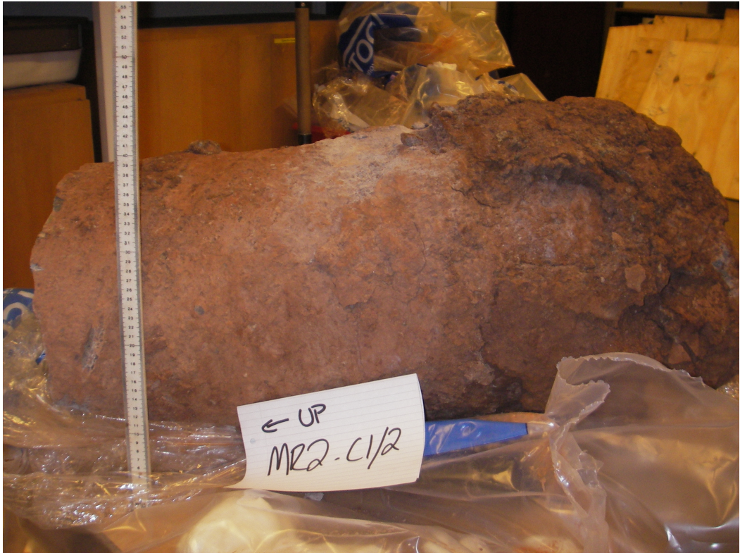
Figure 4.17 The first section taken from pile MR2 0-1000mm below ground level
