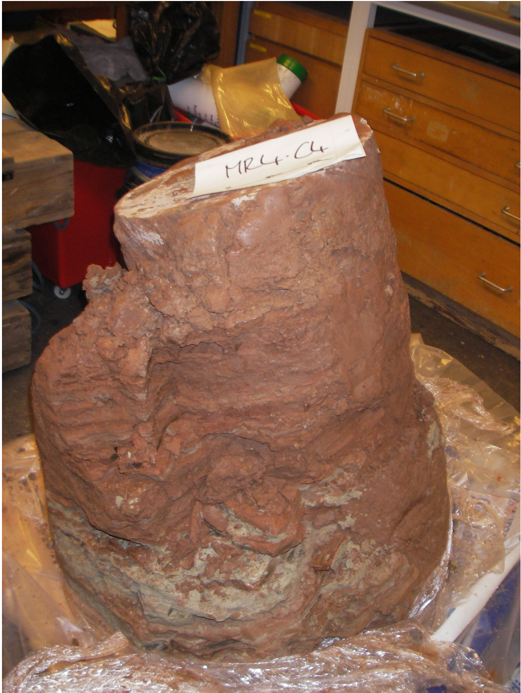
Figure 4.40 The final section taken from pile MR4 1342-1962mm below ground level
