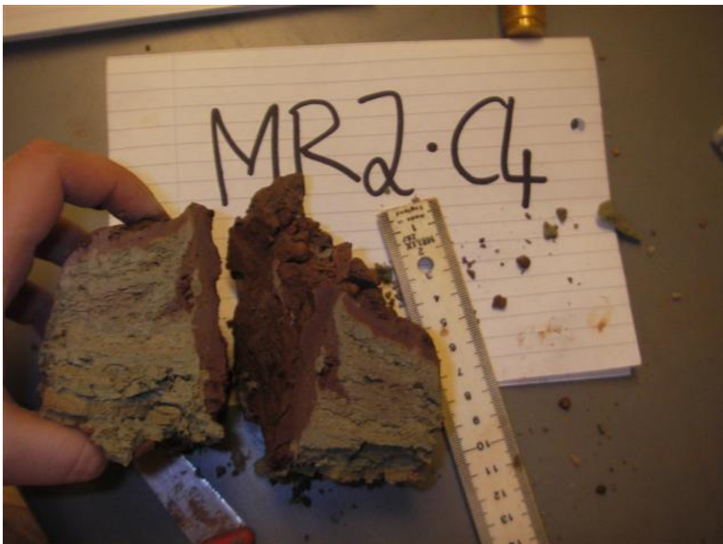
Figure 4.25 The colour change between remoulded and undisturbed material from around pile MR2 at a depth of 1457-1979mm below ground level
