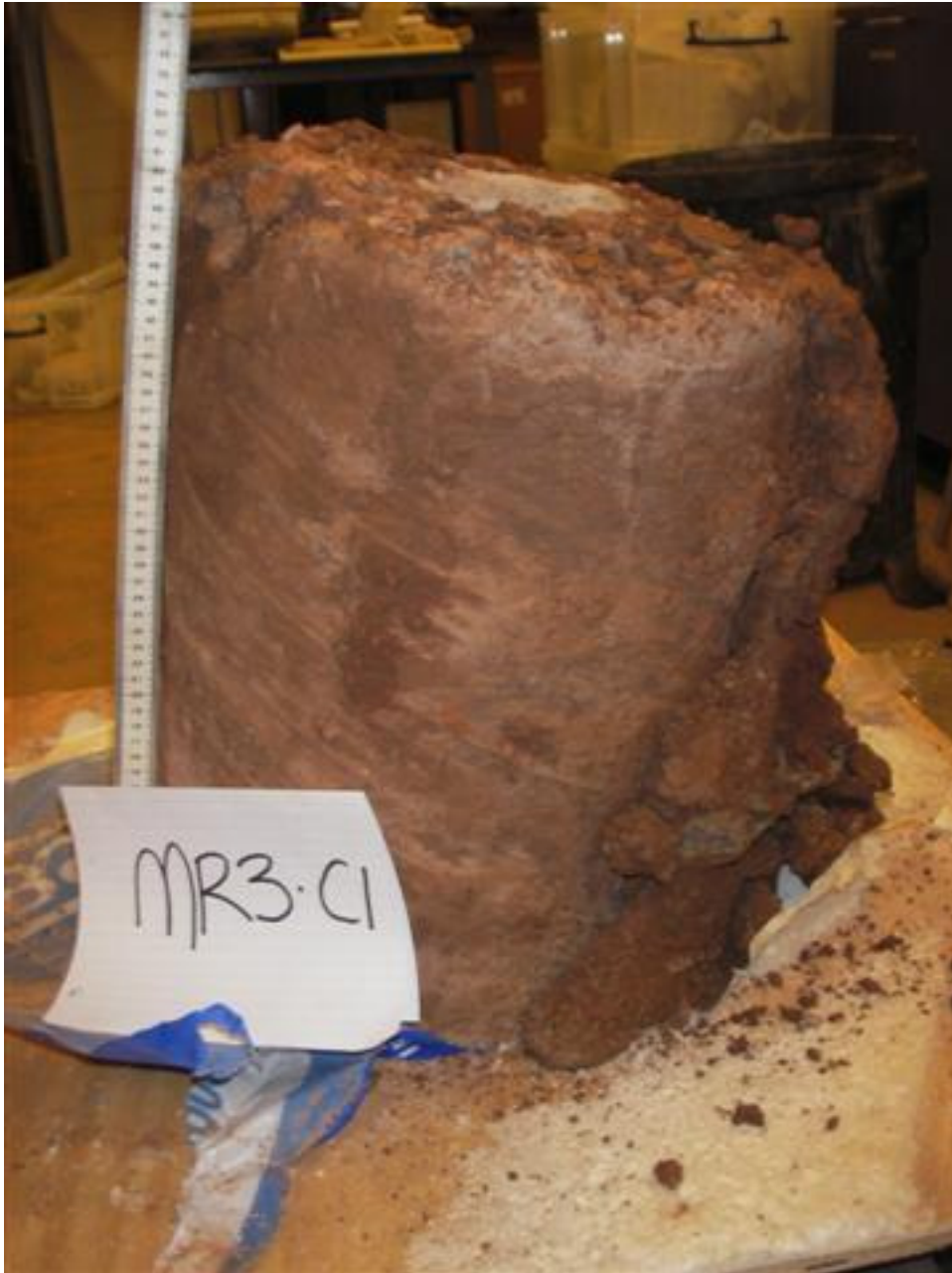
Figure 4.26 The first section from pile MR3 0-510mm below ground level
