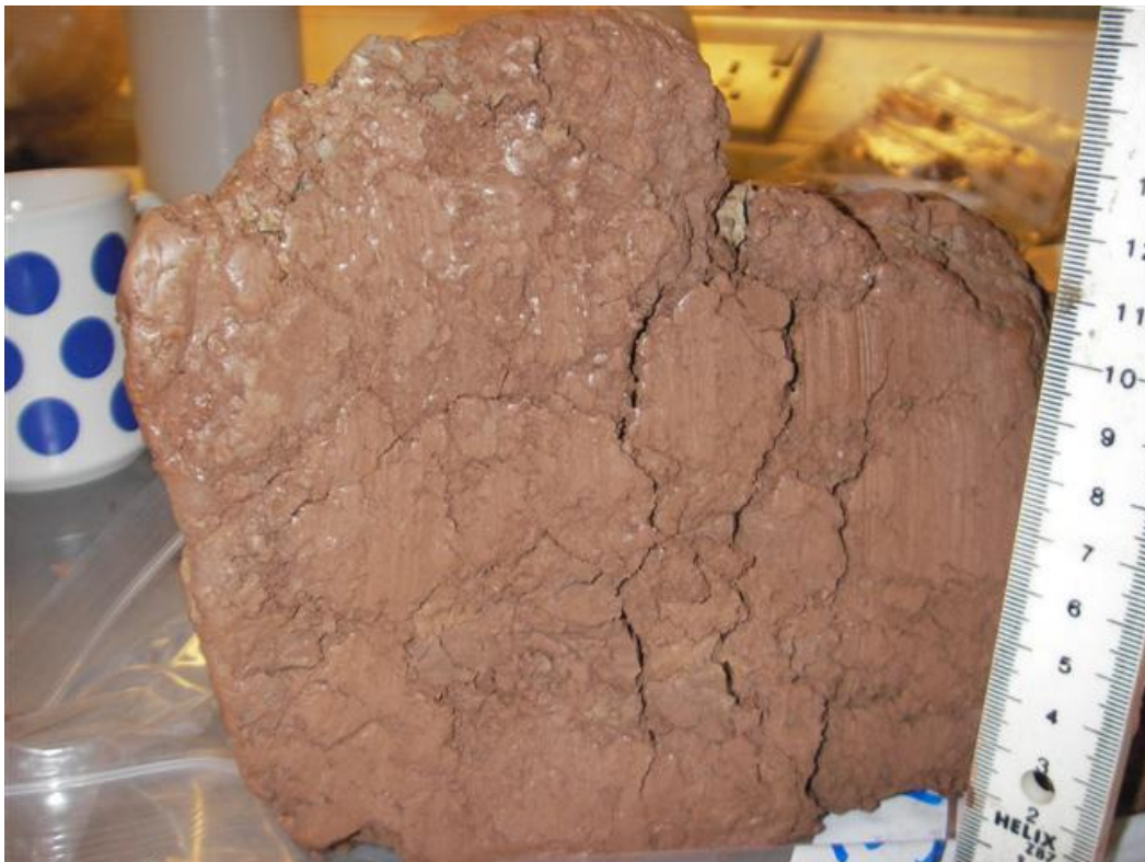
Figure 4.34 The inner surface of the remoulded zone from around pile MR3, 860-1210mm below ground level. Pile would have been to the front of the picture
