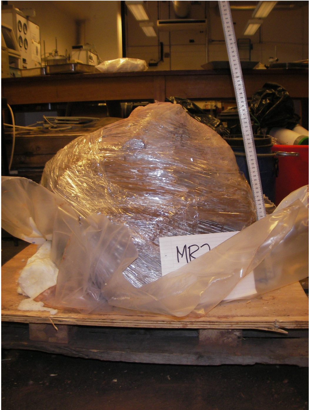
Figure 4.18 The second section taken from pile MR2 1000-1457mm below ground level
