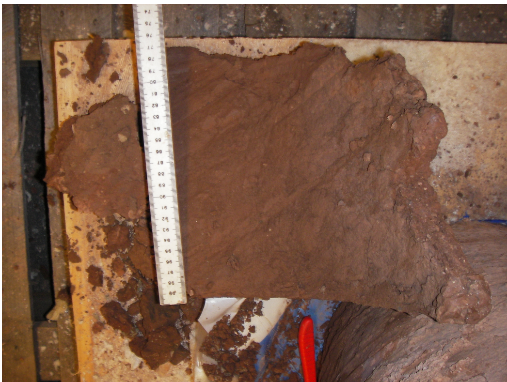
Figure 4.30 The inner edge of the soil-pile interface in the remoulded soil surrounding pile MR3, base of sample is from 860mm below ground level
