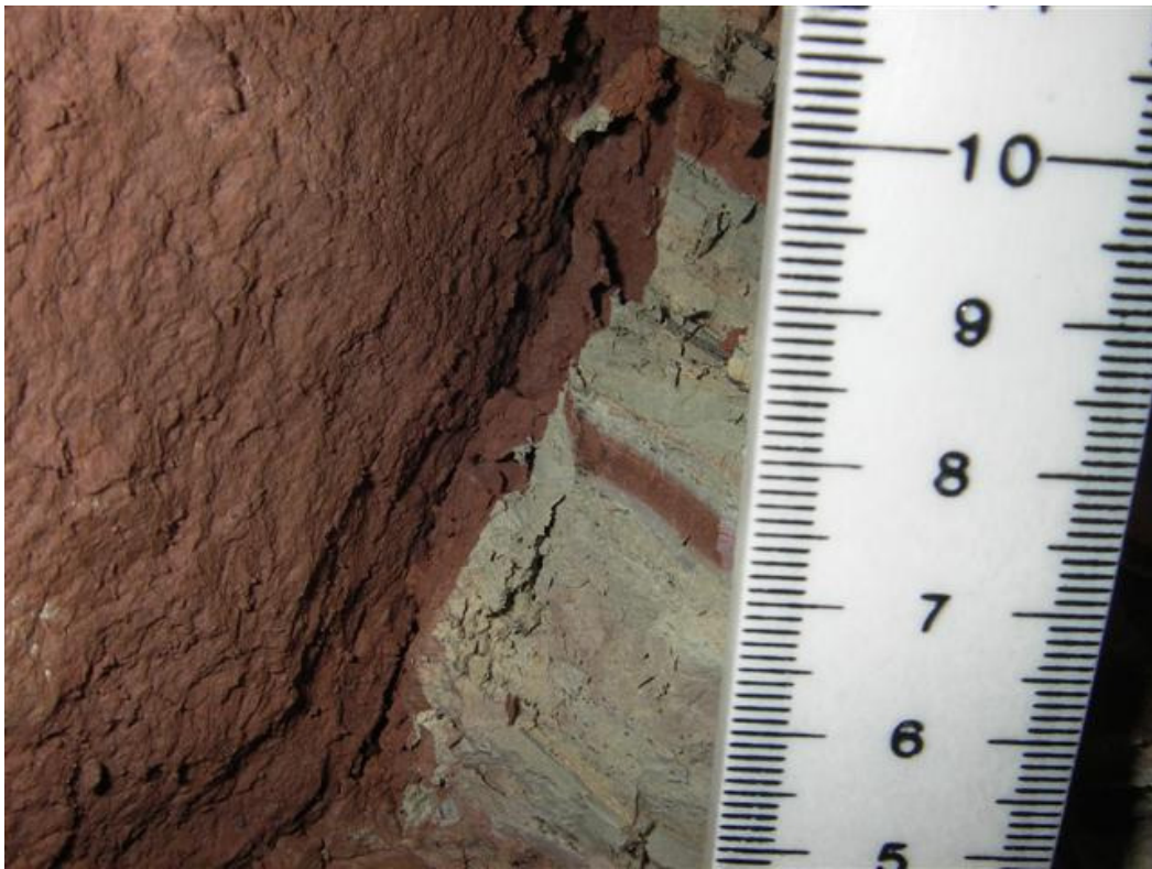
Figure 4.43 The remoulded material from 1600mm below ground level showing the distinct colour and texture differences between the remoulded and host soils
