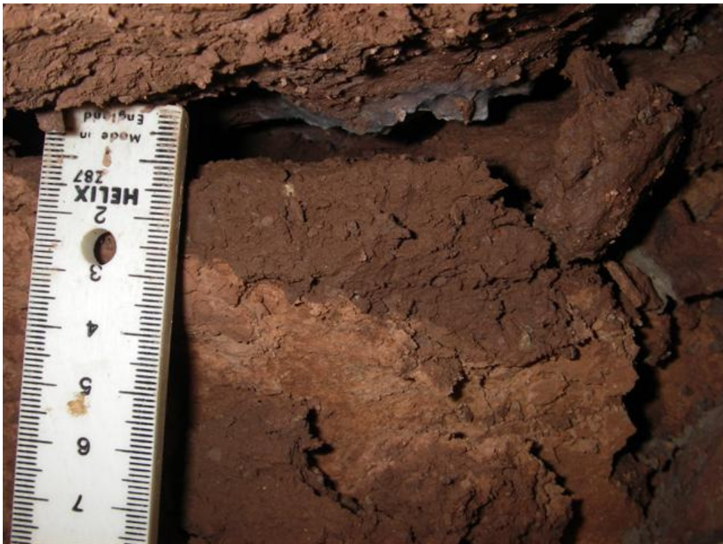
Figure 4.16 The boundary between the host soil and remoulded soil around pile MR1, 819-1277mm below ground level
