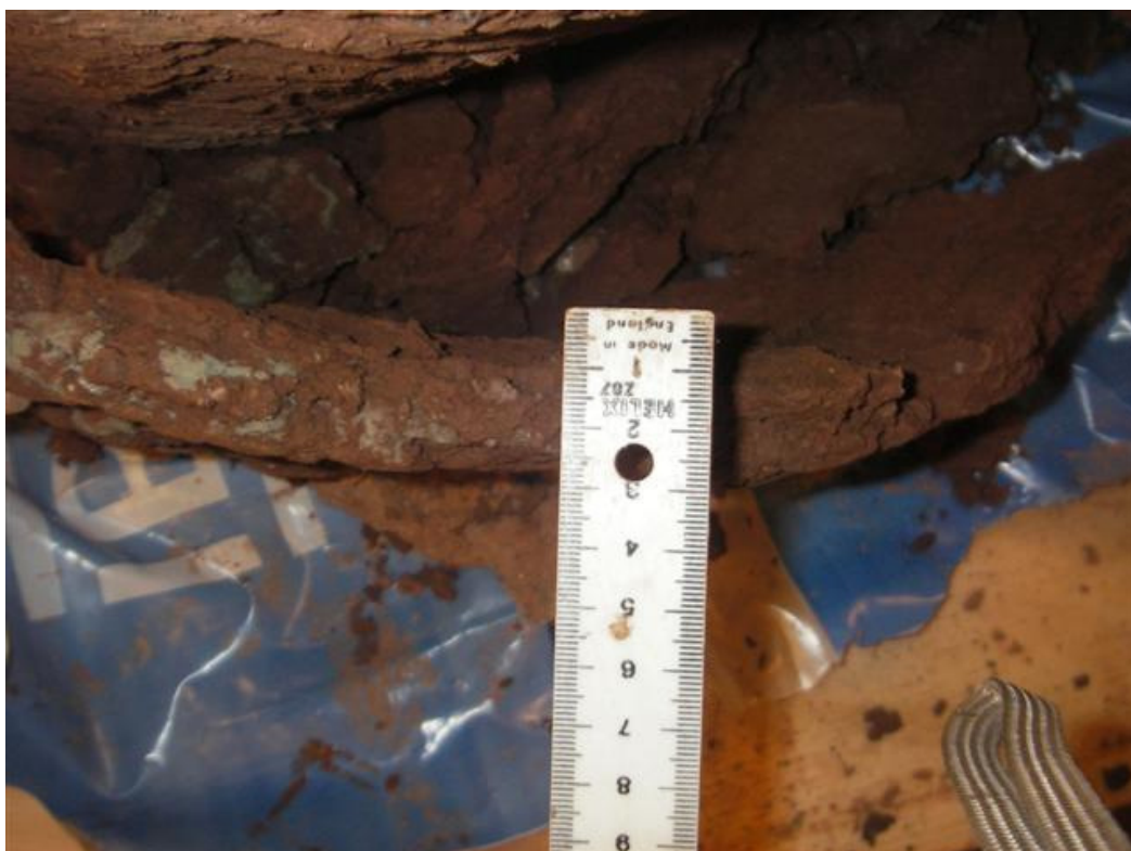
Figure 4.13 Sketch drawing and photograph of remoulded material around pile MR1, 0-495mm below ground level. The photograph is taken looking downwards, with the pile at the top of the picture
