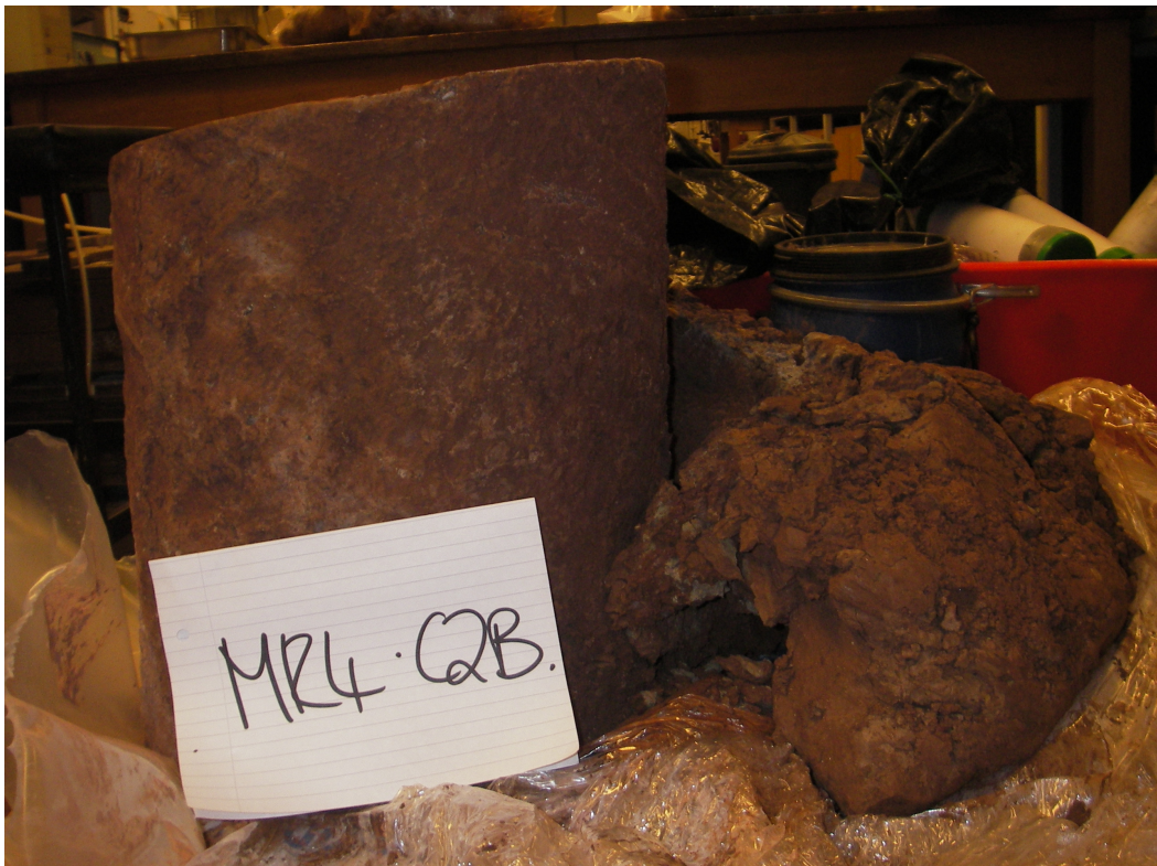
Figure 4.39 The third section taken from pile MR4 951-1342mm below ground level
