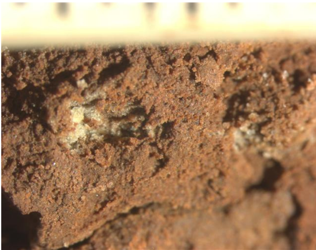
Figure 4.54 The remoulded zone surrounding pile MR4 at 922mm below ground level. Quartz aggregations are seen within this layer. Ruler is in the position of the pile.
