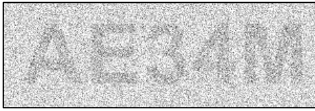
Fig. 16 - Final integrated output result from superimposing 10 CAPTCHA frames shown as an 8-bit/pixel greyscale image. String of "AE34M" can be clearly retrieved by OCR recognition software using CAPTCHA v.1.
