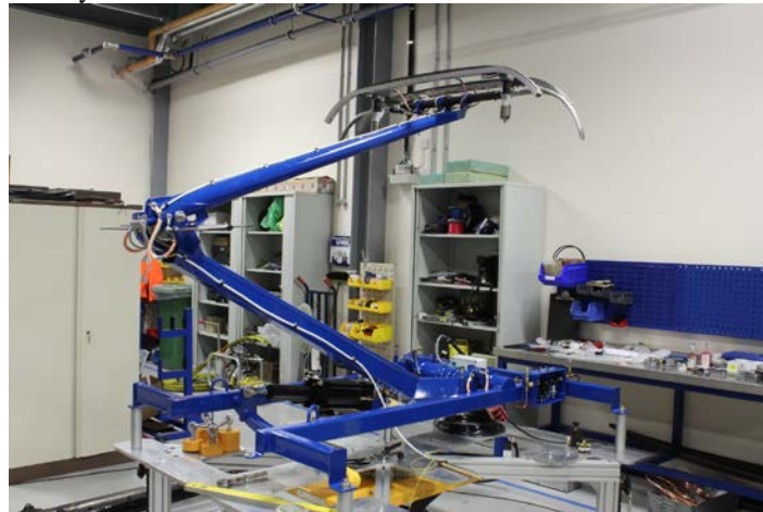
Figure 5. Calibration of a smart pantograph integrated with FBGs in industrial context
