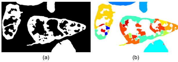
Fig. 6. Example showing over-segmentation caused by the high intra-granular voids using the 3D filling strategy (showing cropped part from Fig. 7(a)): (a) binary image after being filled; (b) segmented image
