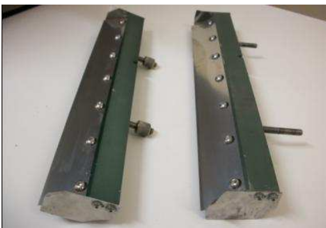
Figure 4.8: Squeegee design used throughout the printing trials
