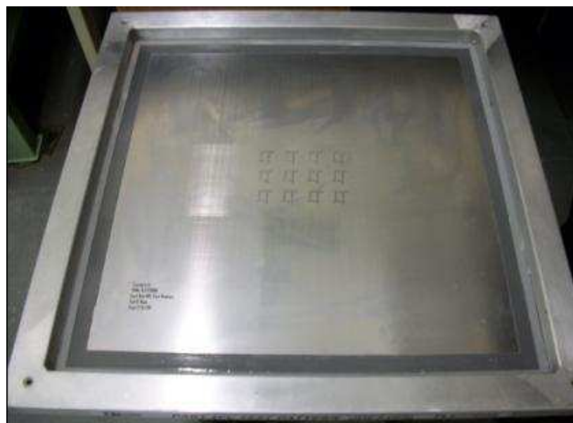
Figure 4.10: IPC slump stencil IPC-A-21
