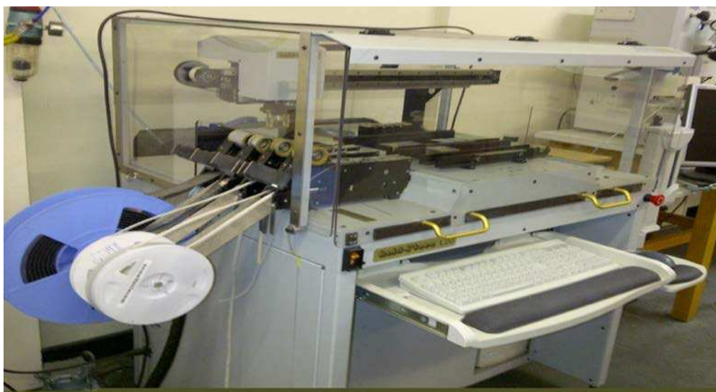
Figure 4.6 Pick and place machine (Gold-Plea L20).
