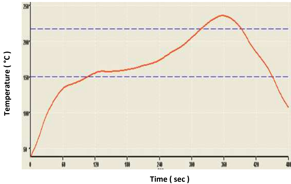
Figure 7.5c Optimal reflow for ( \varnothing 4.3mm) solder bump
