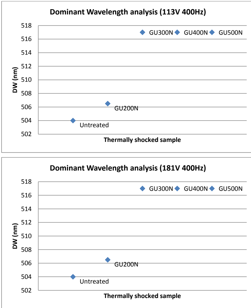
Figure 4.3: Dominant emission wavelength of the nitrogen shock treated samples at (113V and 181V) under 400Hz frequency compared to that of an untreated sample. Dominant wavelength is shifted toward a longer wavelength.
