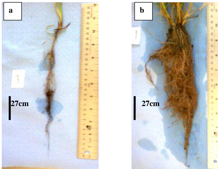
Fig.3.12: Root shape of tall fescue after growing in clean (a) and HC-treated (b) sand for 14 months
