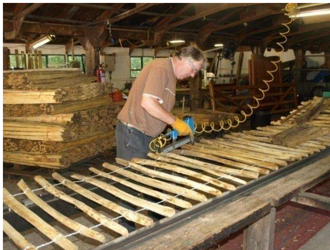
Figure 4.7 Flat bed paling system showing stapling of the wire to the pales
