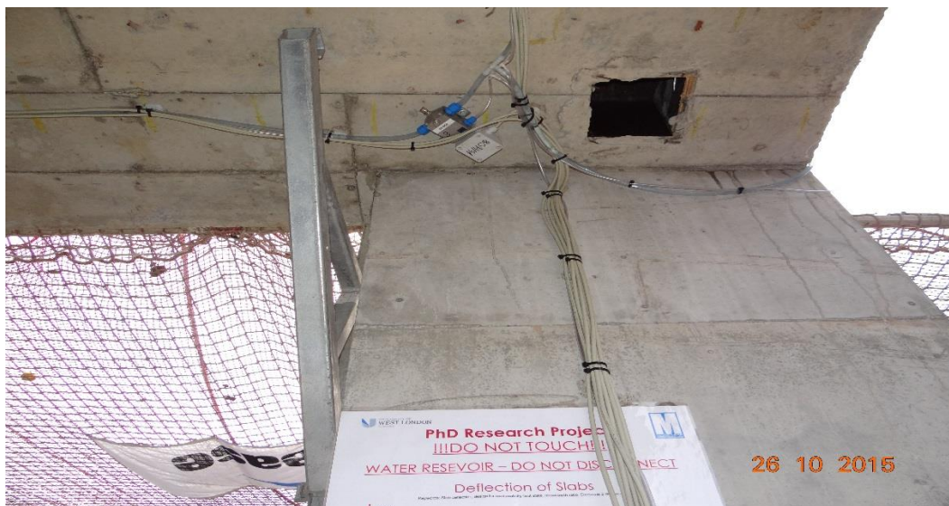
Figure 3.7 Hydraulic Cell Level Network Connection
