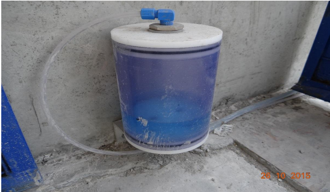
Figure 3.8 Hydraulic Cell Level water pressure reservoir
