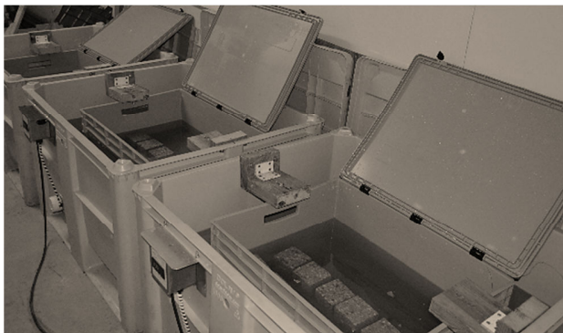
Fig. 1 Experimental set up of cubes being submerged into diluted sulphuric acid
