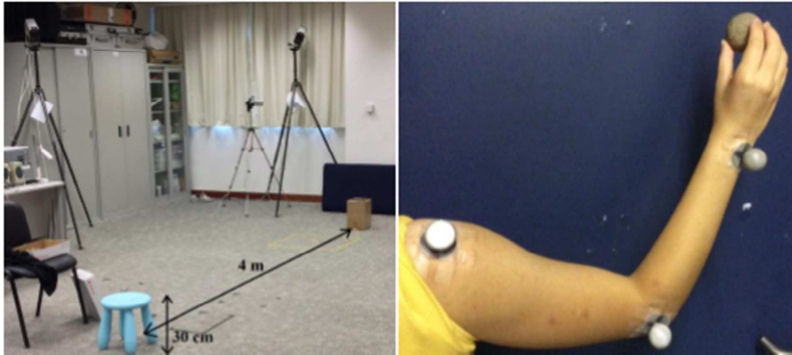
11 12 13 14 15 16 17 18 19 20 21 22 23 24 25 26 27 28 Fig. A1. (Left) The experimental setup showing the 30cm high stool, the smallest target box and 2 of 29 the Qualysis cameras. (Right) The markers on shoulder and elbow (acromion- and olecranon process) 30 and wrist (radial styloid) as well as the hand (reflective golf-ball). 31 32 33 34 35 36 37 38 39 40 41 42 43 44 45 46 47 48 49 50 51 52 53 54 55 56 57 58 59 60
