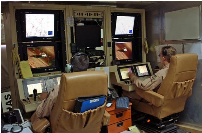
Figure 2: MQ-1 Predator Control Station. Source: http://www.af.mil/shared/media/photodb/photos/070807-F-9602H-101.jpg
