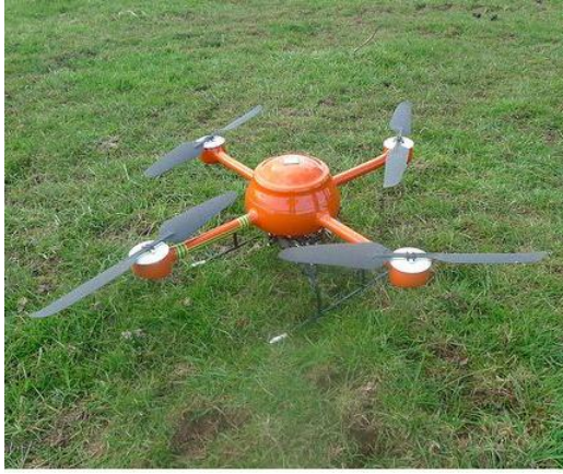
Figure 5.2a: Microdrone MD4-200 helicopter.
