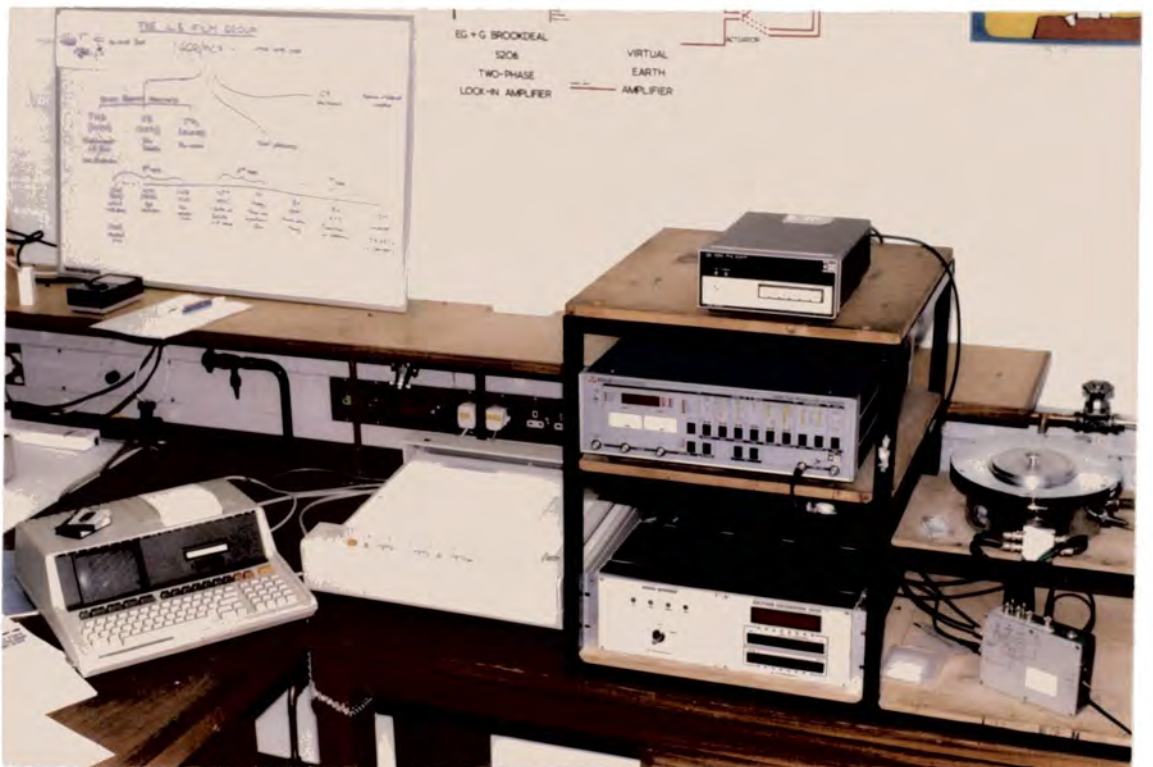
Figure 4.16 : Instrumentation arrangement for automated a.c. admittance measurement
