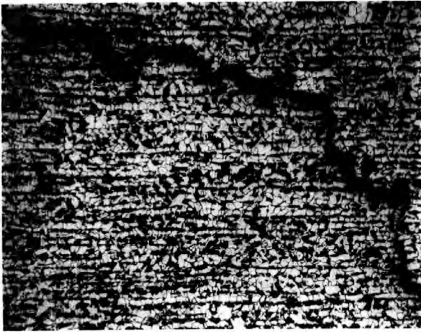
Figure 106 Metallographic section of pipe section 3 showing extent of banding x 200
