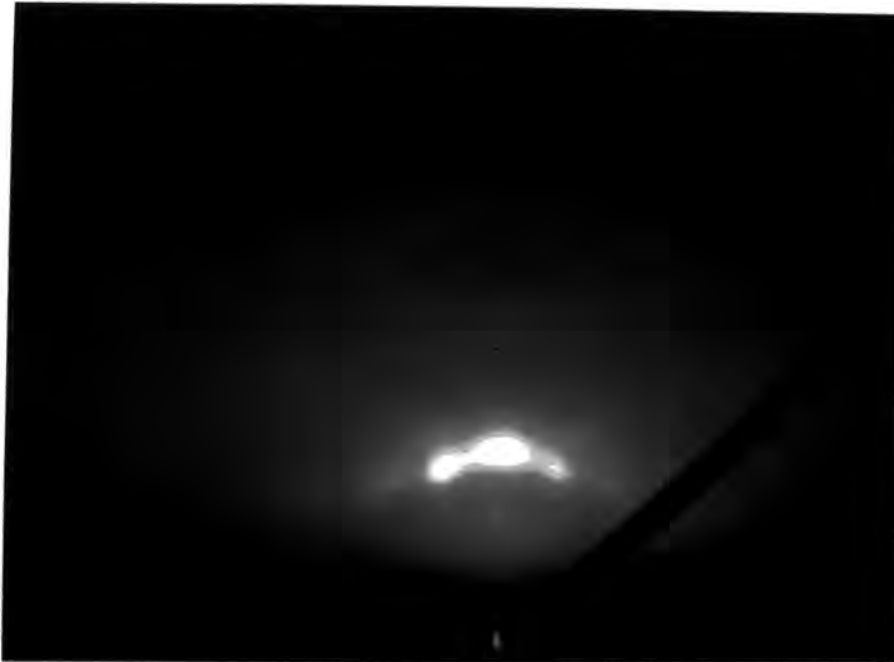
Figure 5.12 RHEED pattern from 3 layer film of 22-TA on hydrophilic silicon surface.
