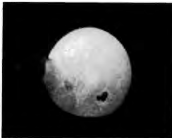
Figure 5.17 Spatial distribution of EL from a ZnSe MIS diode with an epitaxial ZnS I-layer (actual contact diameter 1.5 mm).
