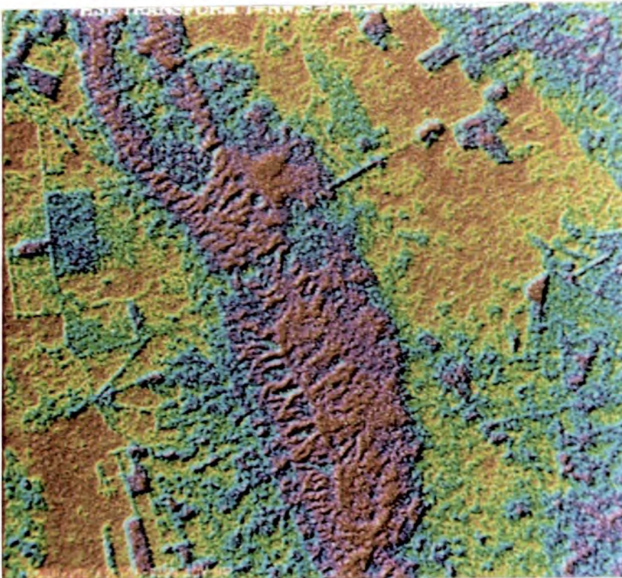
Plate 5.55 HSI transform of the filtered SIR-A image of Djebel Cherahil. Hue is determined by the low-pass filter, saturation by the high-pass filter and intensity by the directional filter. The image is valuable for revealing textural information and linear features.
