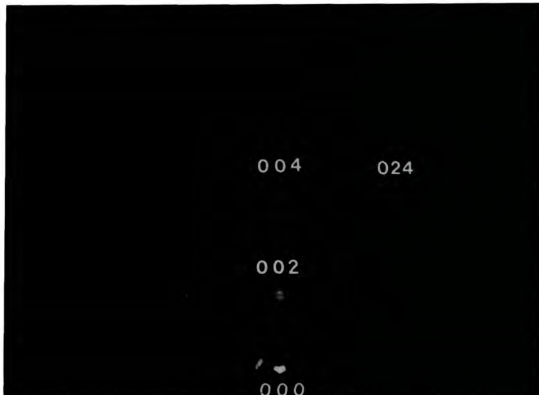
Figure 8.6: RHEED pattern from Cr/MgO single crystal; dopant concentration 800ppm, etching time 1 min.
