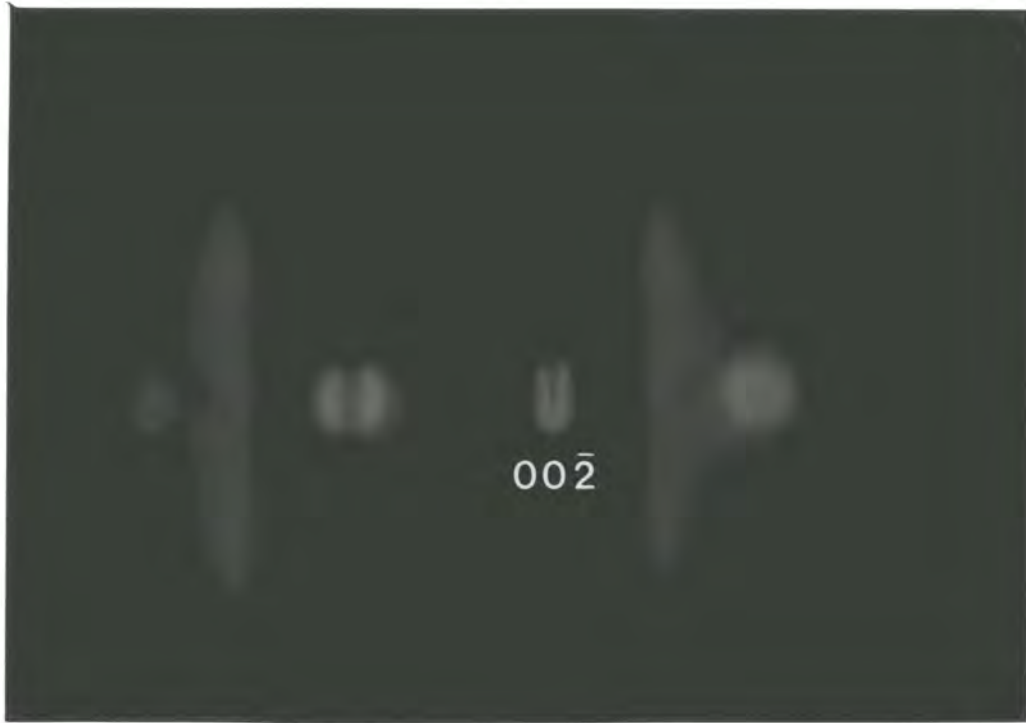
Figure 3.10d Microdiffraction pattern (CL=20cm) showing destructive interference through a \{200\} disc due to interaction with a pair of doubly diffracted \{9\ 1\ 1\} , \{11\ 1\ 1\} reflections:- taken from the CdTe substrate of an MCT/ \{111\} CdTe sample which gave good MCT growth.
