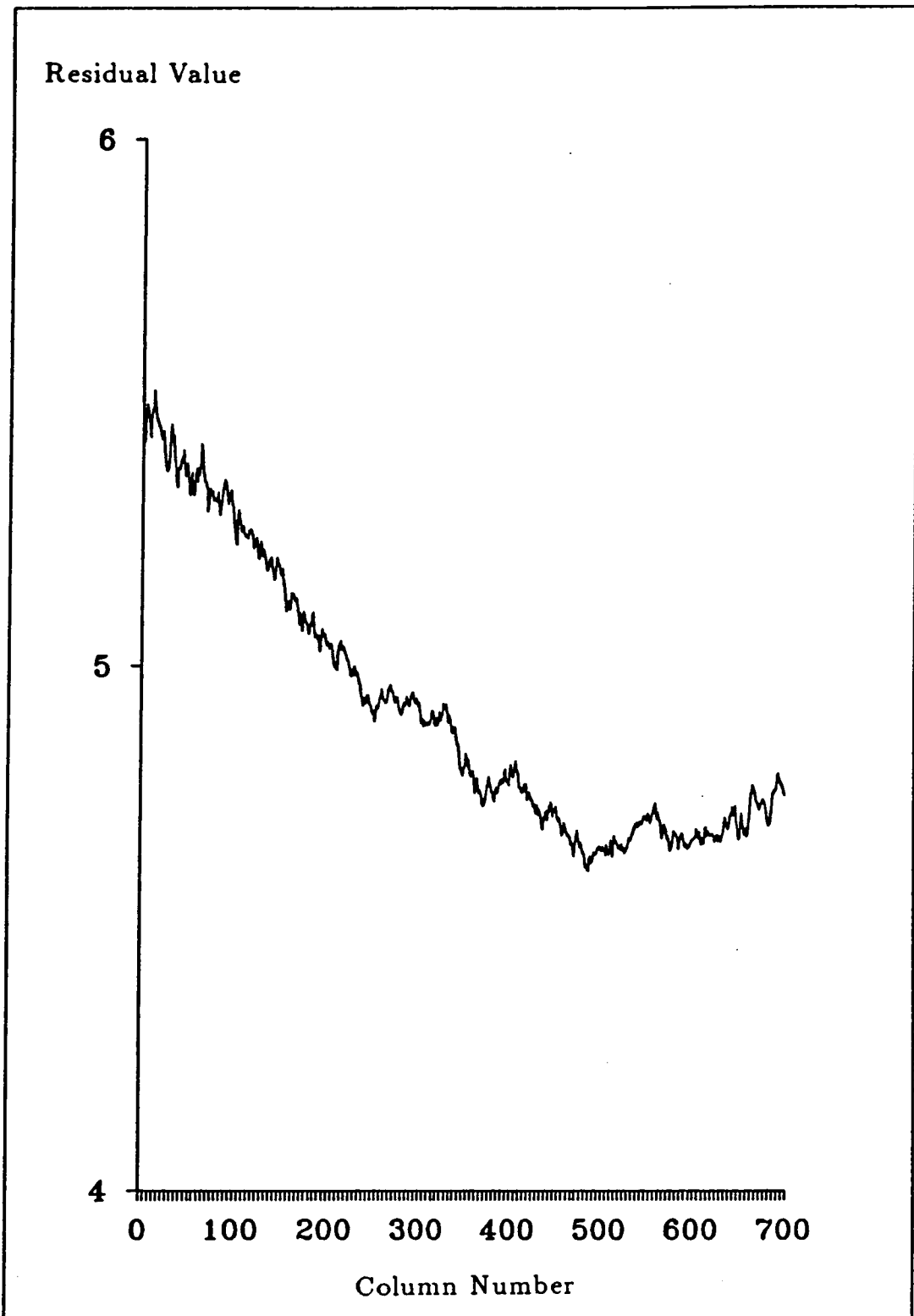
Figure 3.8 Residual Curve from Dividing NS-001 Column Means of Channel Six by Channel Seven, Flightline 1.
