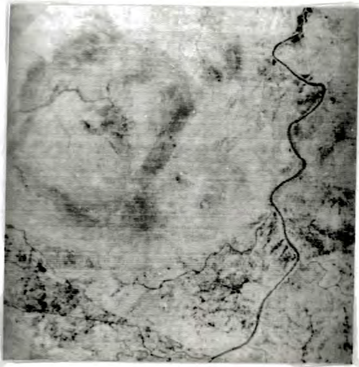
Plate 5.11 Thermal Log Residual of the 8.8\mu\text{m} Channel, Camp Oven Test Site.
