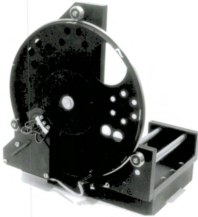
Figure 4.3: Aperture wheel assembly.
