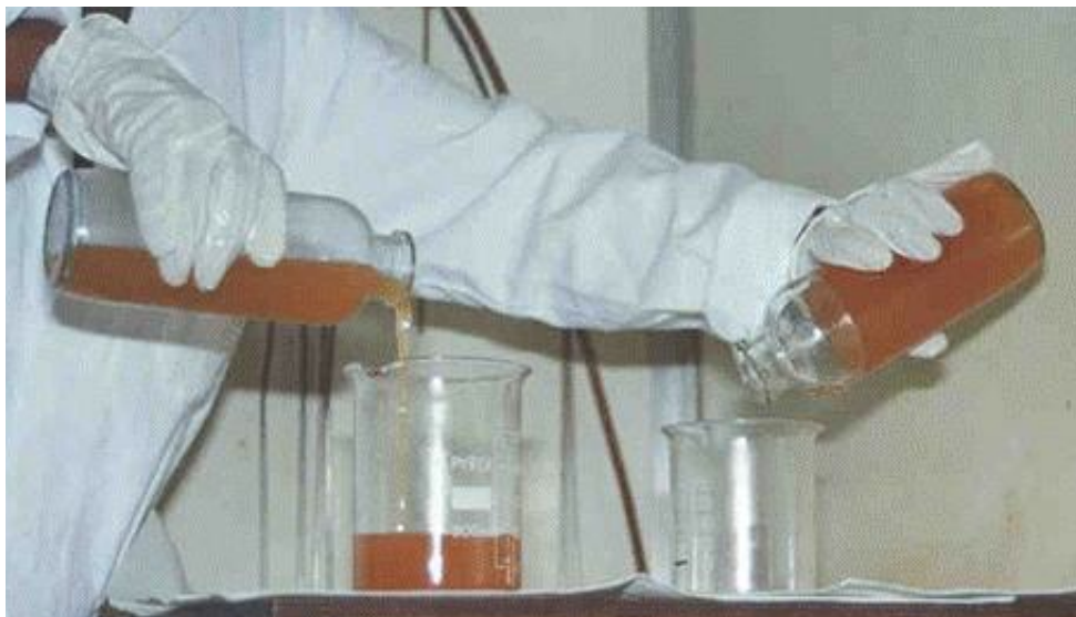
Figure 1.2: The pouring properties of base fuel, without (right) and with (left) additive, cooled overnight to minus ten degrees Celsius, picture provided by Infineum.
