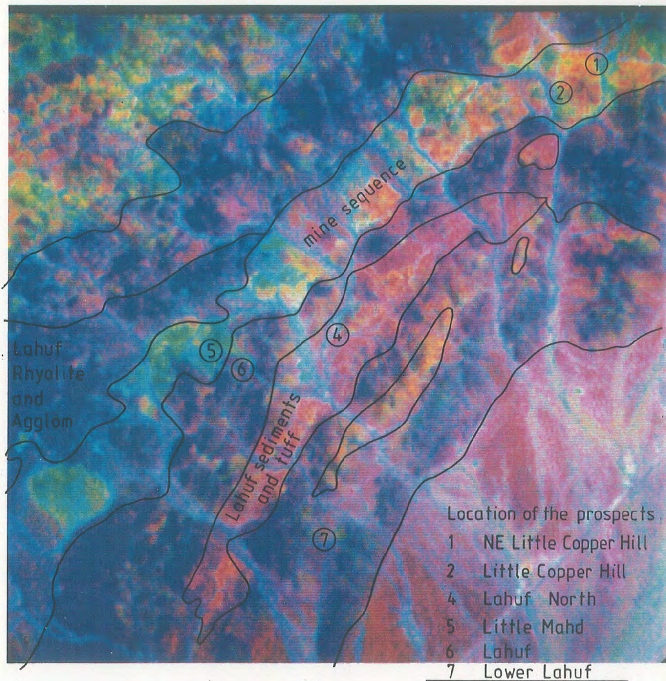
Fig. 6.21 The west of Mahd Adh Dhahab Mine (see Fig. 6.17 for location). Zoom over the mine sequence and other lithologies. Decorrelation stretched image 7,5,2 in R.G.B show the location of the prospects (see Table 6.2).
