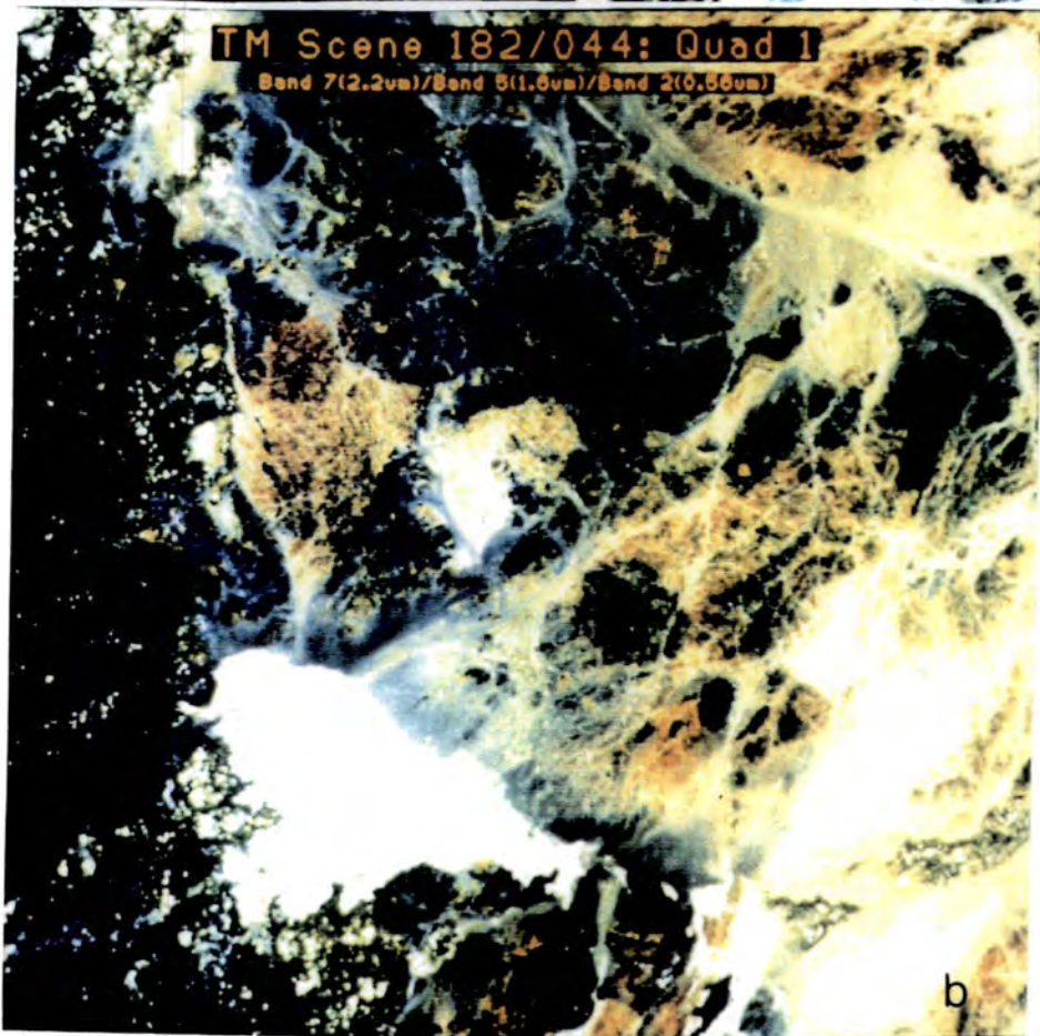
Fig. 6.2 a. Simulated true colour of TM using band 3.2.1. Image cover both areas Mahd Adh Dhahab and Jabal Said. b. TM False Colour Composite using bands 7, 5 and 2 in RGB respectively.
