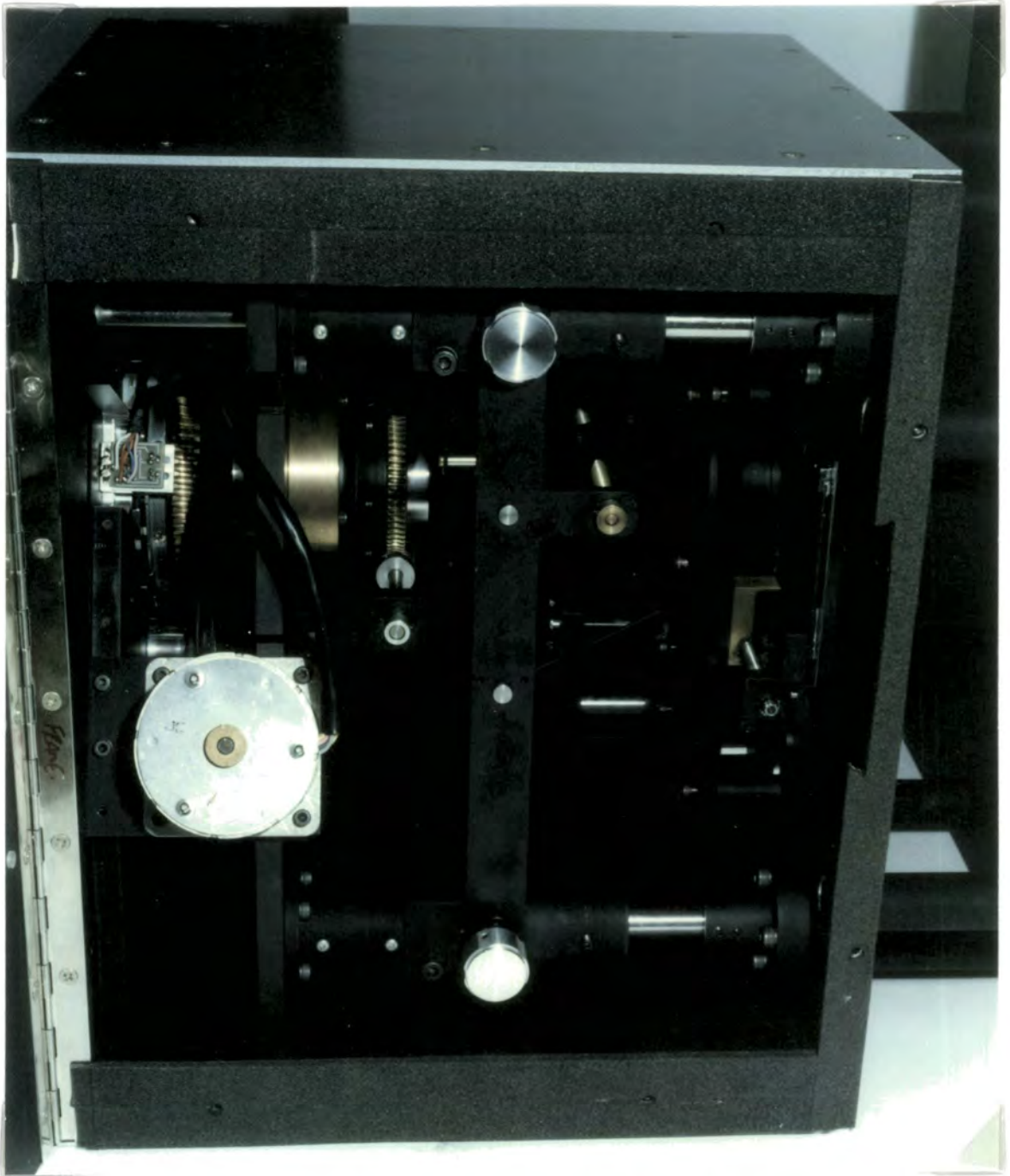
Figure 1.2: The Durham Imaging Polarimeter. The optical and mechanical components are closely packed inside a light-tight case; the grid assembly runs in the dovetail slot on the right of the picture, and the relay lens is to the extreme left.
