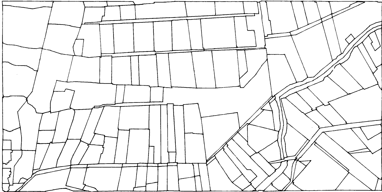
6.46 An overlay of the 1:50,000a coverage and the 1:50,000b coverage following an ELIMINATE of AREA/PERIMETER: 25 units
