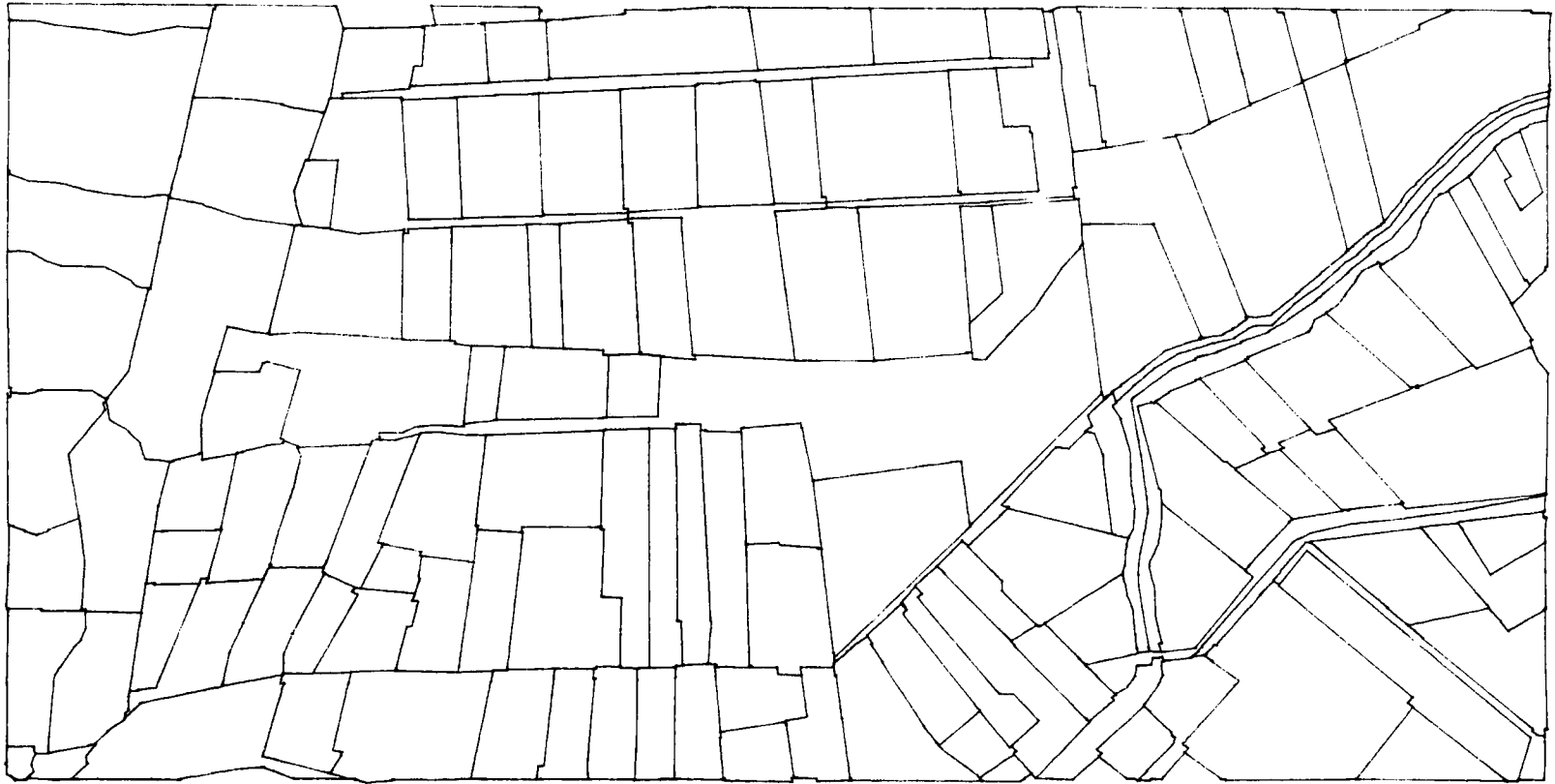
6.39 An overlay of the 1:50,000a coverage and the 1:50,000b coverage following an ELIMINATE of AREA: 8,000 units
