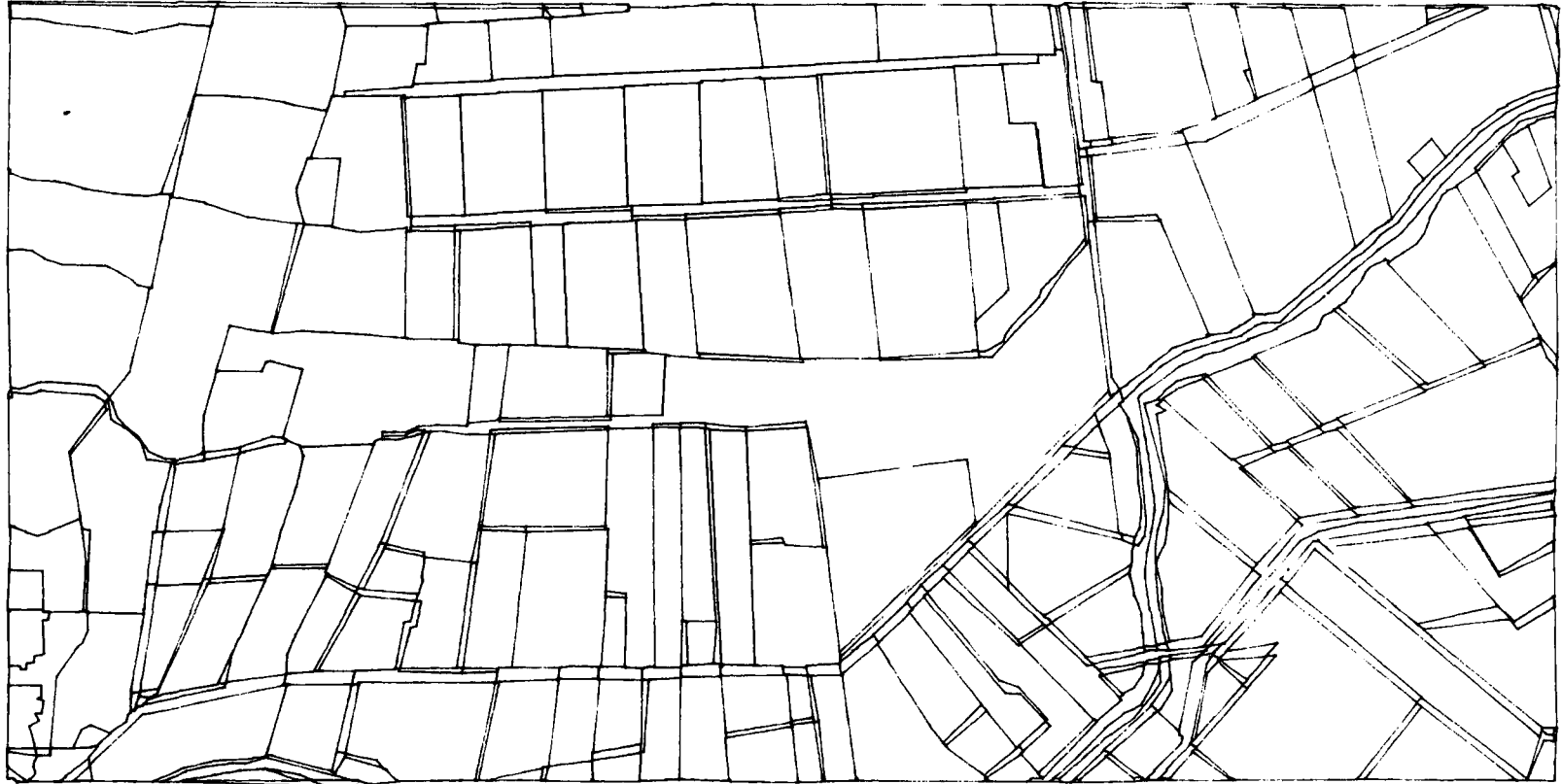
6.42 An overlay of the 1:50,000a coverage and the 1:50,000b coverage following an ELIMINATE of AREA/PERIMETER: 10 units
