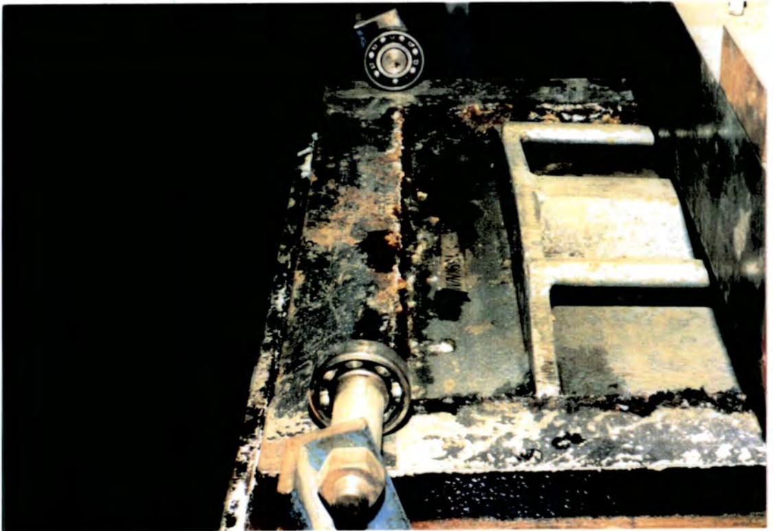
Plate 6.10: Crystalline growths around box lid observed during large shear box test (Gale Common 5 year weathered shale).
