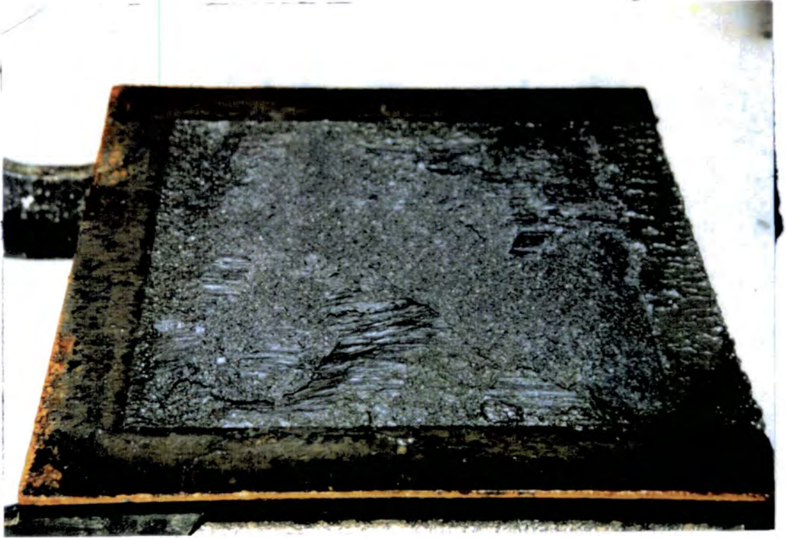
Plate 6.5: Shear plane from large shear box test (fresh Coal Measures shale passing 2mm sieve).
