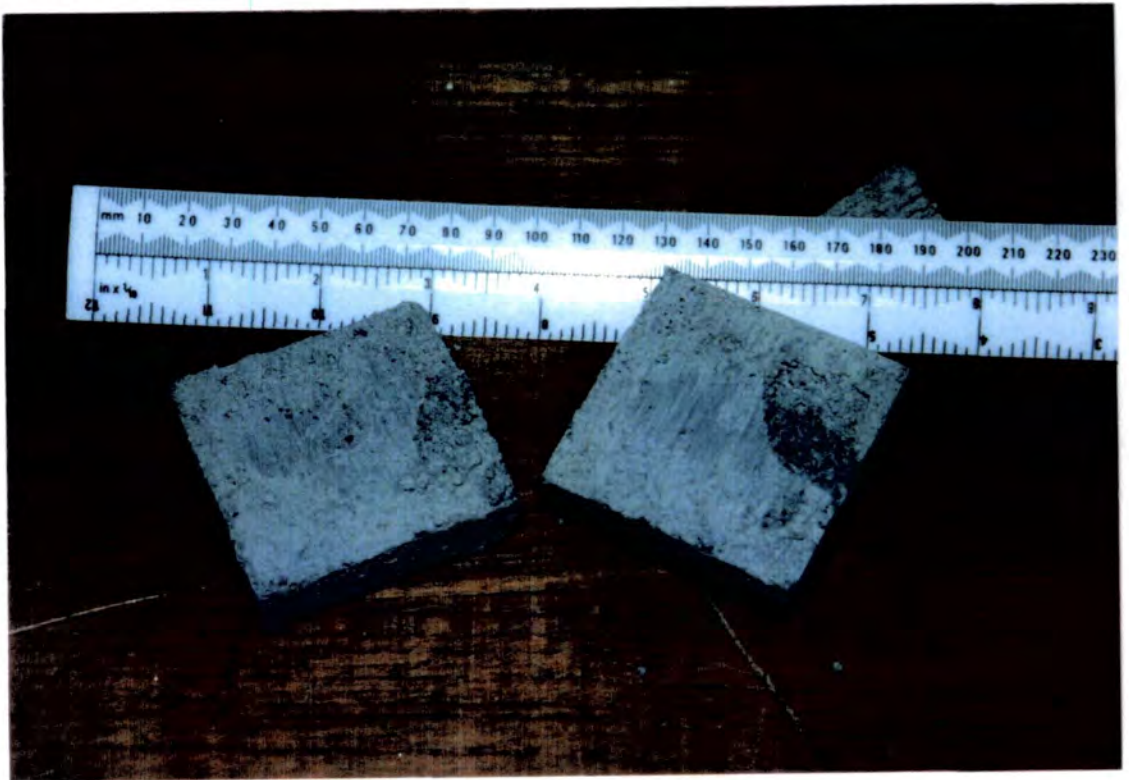
Plate 6.4: Sample from small shear box split after testing to reveal shear plane (Coal Measures shale passing 2mm sieve).
