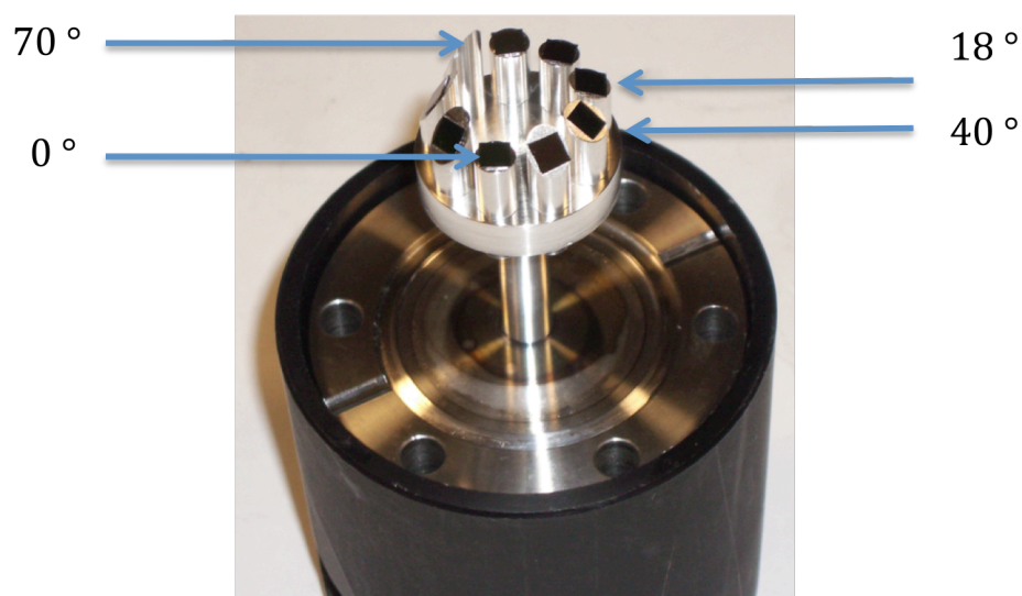
Figure 27. Thermal evaporator sample holder - that can hold samples between the angles of 0 ° and 70 °. The four angles used throughout this study are highlighted on the sample holder. The sample holder is held at the top of the thermal evaporator chamber.
