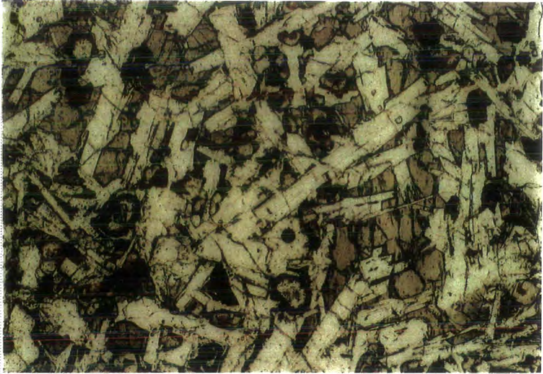
Photo: 6.10. Microphotograph of the subophitic Karapmar basalt, sample MK289, base of the volcanic sequence, Mt. Kargapazarı. Magnification 4x, PPL.
