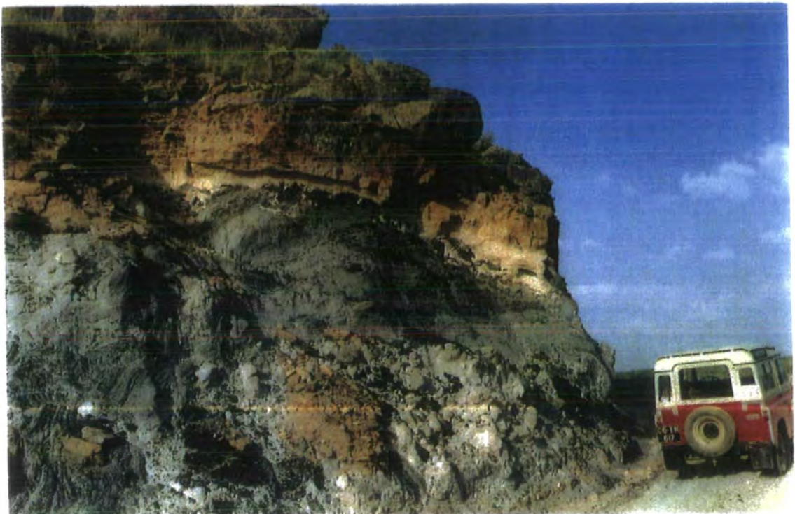
Photo: 2.20. Field photograph showing the sharp contact between the Grey (Gign) and Black ignimbrite (Bign), N of Malikom village (P:33), NW of Pasinler.
