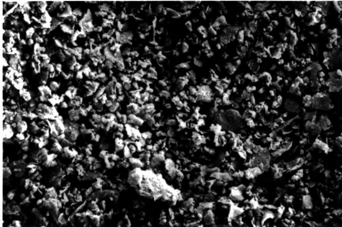
Figure 7.4.3 SEM of sample WM4 after 40 days laboratory weathering at pH 6.0. The mineral grains have taken on the 'woolly' weathered appearance similar to that in figure 7.1.2. (x500; WD 7 mm; 1 cm = 15 \mu m)
