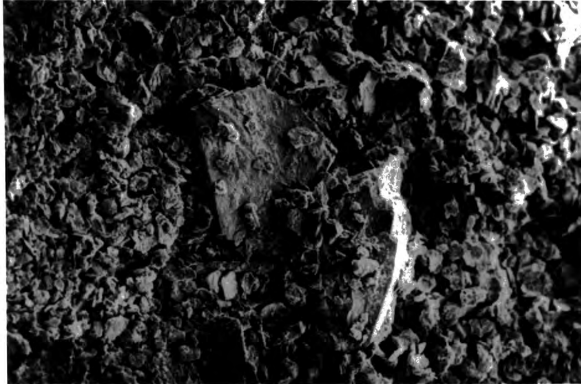
Figure 7.1.1 SEM of sample WM5, an example of clean grains, unaffected by chemical weathering or clay coating. (x500; WD 7 mm; 1 cm = 15 \mu m)
