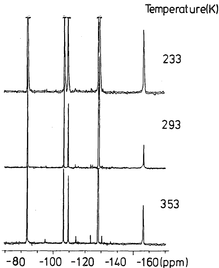
Figure 4,6. ^{19}\text{F} -NMR spectra of the carbanion(141) at various temperature. Solvent : \text{CD}_3\text{CN}
