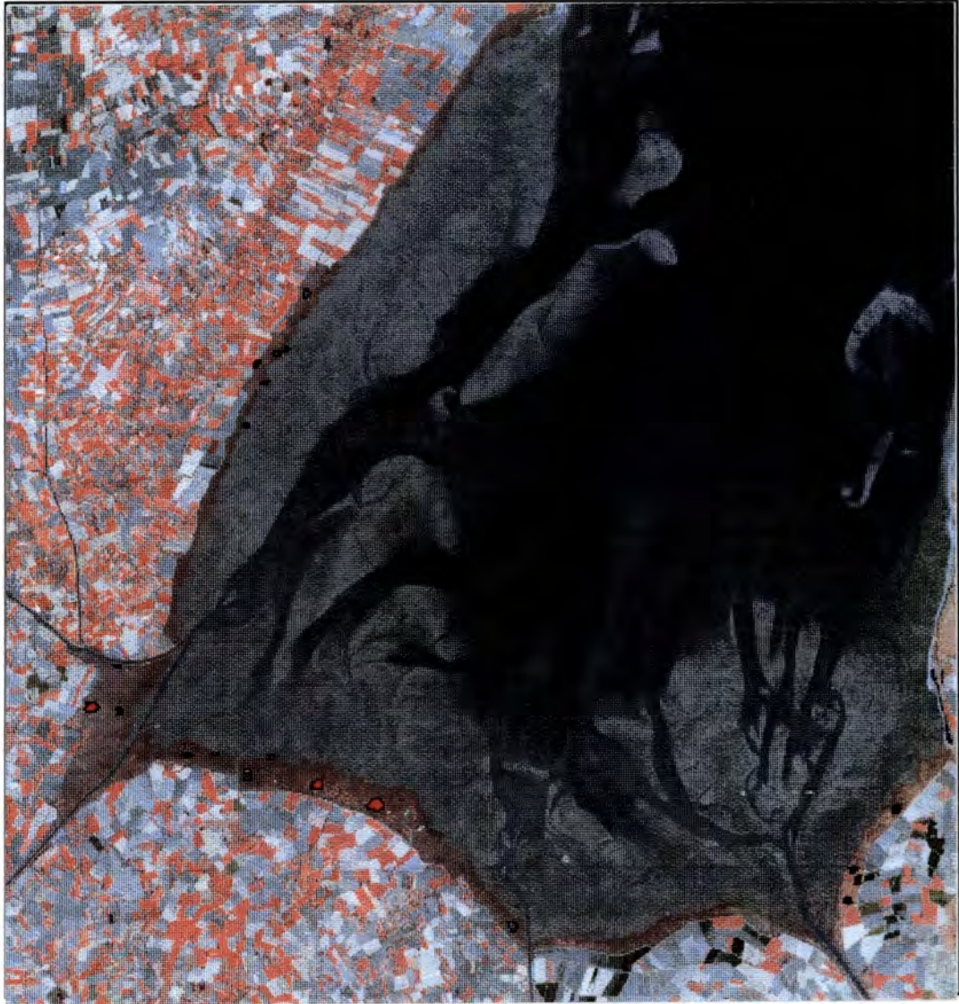
Fig. 6.3 Location of training areas on the September 1991 Landsat5 TM image (operator 2). (red = TM4, green = TM3, blue = TM2).
