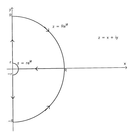
Figure 5.4. The two paths (one in the upper quadrant, one in the lower) around which the integral  $\oint z^{n+1} e^{-z} dz$  is evaluated in order to evaluate  $\int_0^\infty x^{n+1} \sin(x) dx$ .
