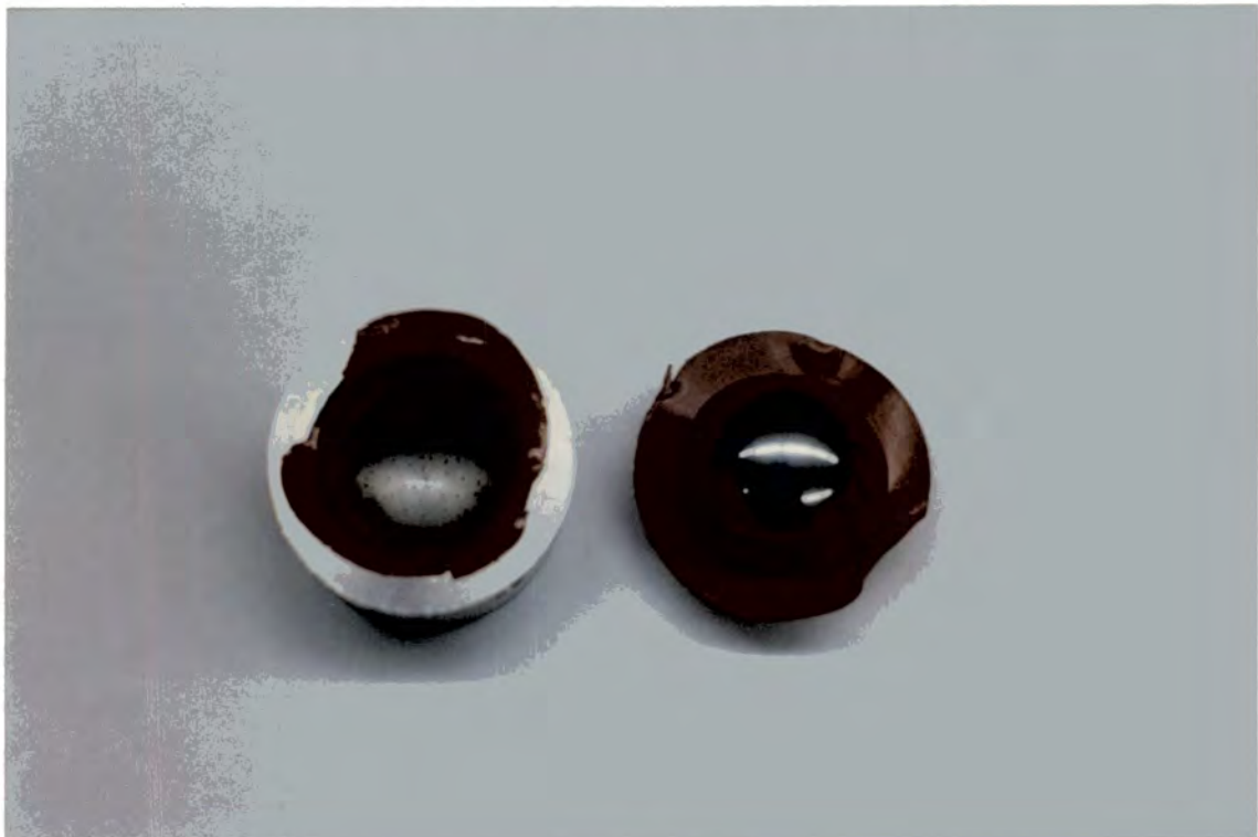
Figure 6.8 : Typical Silicone Rubber Mouldings from Loaded Prosthetic Devices
