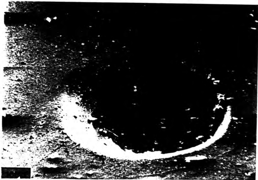
Figure 7.6b : Pore ablation at 4mJ in Tecoflex 93 o A showing poor hole formation
