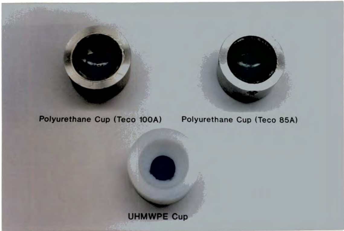
Figure 6.7 : Typical Dyed Regions from Loaded Prosthetic Devices
