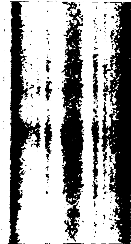
Fig. 2.8: Experimental section topograph of a perfect crystal, showing an undistorted set of Pendellösung fringes.
