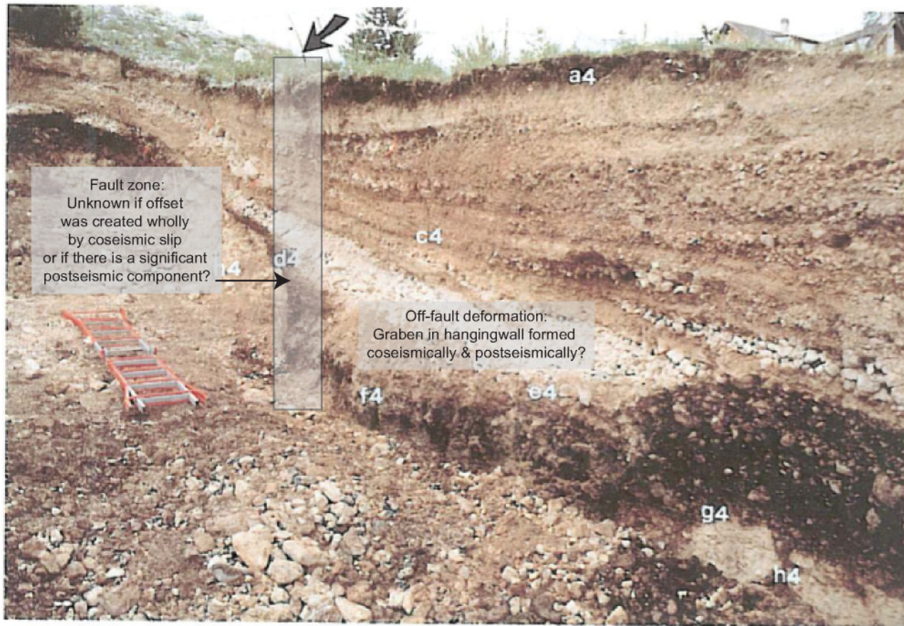
Figure 6.2.4: The trench wall of a paleoseismic study of the Ovindoli-Pezza normal fault in the central Apennines [D'Addezio et al., 1996]. The fault zone is denoted by the arrow. Note the graben which has formed in the hangingwall. The proximity of the graben, off-fault deformation to the fault zone makes it difficult to precisely distinguish on-fault coseismic offsets from off-fault postseismic deformation in such studies.
